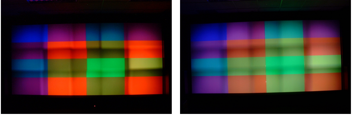
Figure 1: Left: A Display of a 5 \times 3 array of 15 projectors where the overlap regions are blended by using a physical shadow mask on the light path of the projector. Right: Same display with the overlap region blended by a linear ramp in software. For this, one needs to know the exact location of the overlap region. Note that the projector boundaries are noticeable in both cases.
