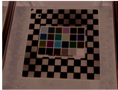
Figure 6. The geometric and photometric calibration patterns, as seen from one of the eight cameras. The patterns shown together here are actually used separately for geometric and photometric calibration.
