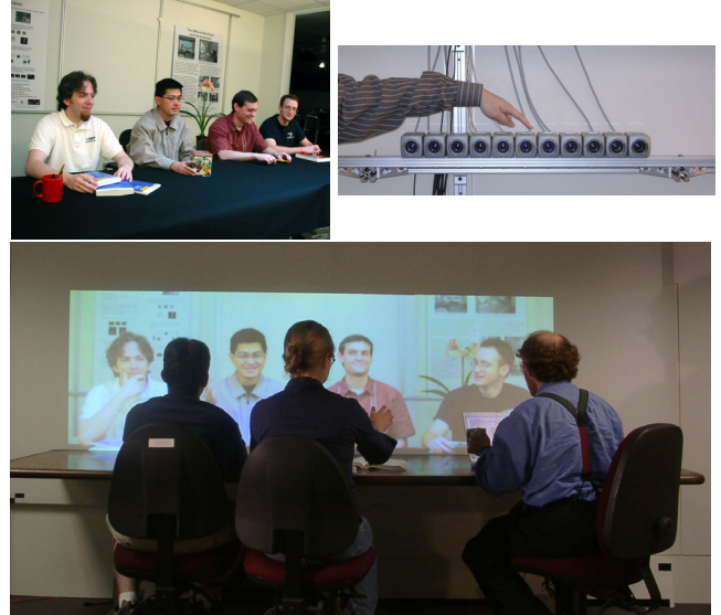
Figure 1: Our Multiple-Camera Group Video Teleconferencing Prototype in Use: The top photo left shows the remote participants. Our camera array to capture the participants is shown in top right. The bottom photo shows the local participants. The life-size, seamless image is synthesized using our method in Section 3.
