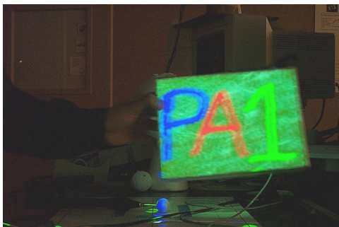
Figure 3: Demonstration of the latency in the tracking pipeline. Notice the blurring and trails artifacts.
