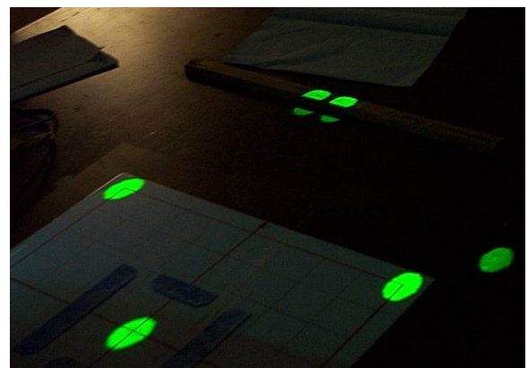
Figure 6: Verification of calibration - drawing markers at known positions in the real world using calibration matrices. When the calibration is a little off, this method can be used to detect this and roughly recalibrate by moving the projector until the images all snap to the correct locations.
