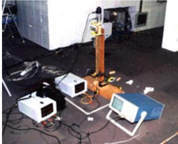
Figure 2-4. Device constructed for measuring system lag.
