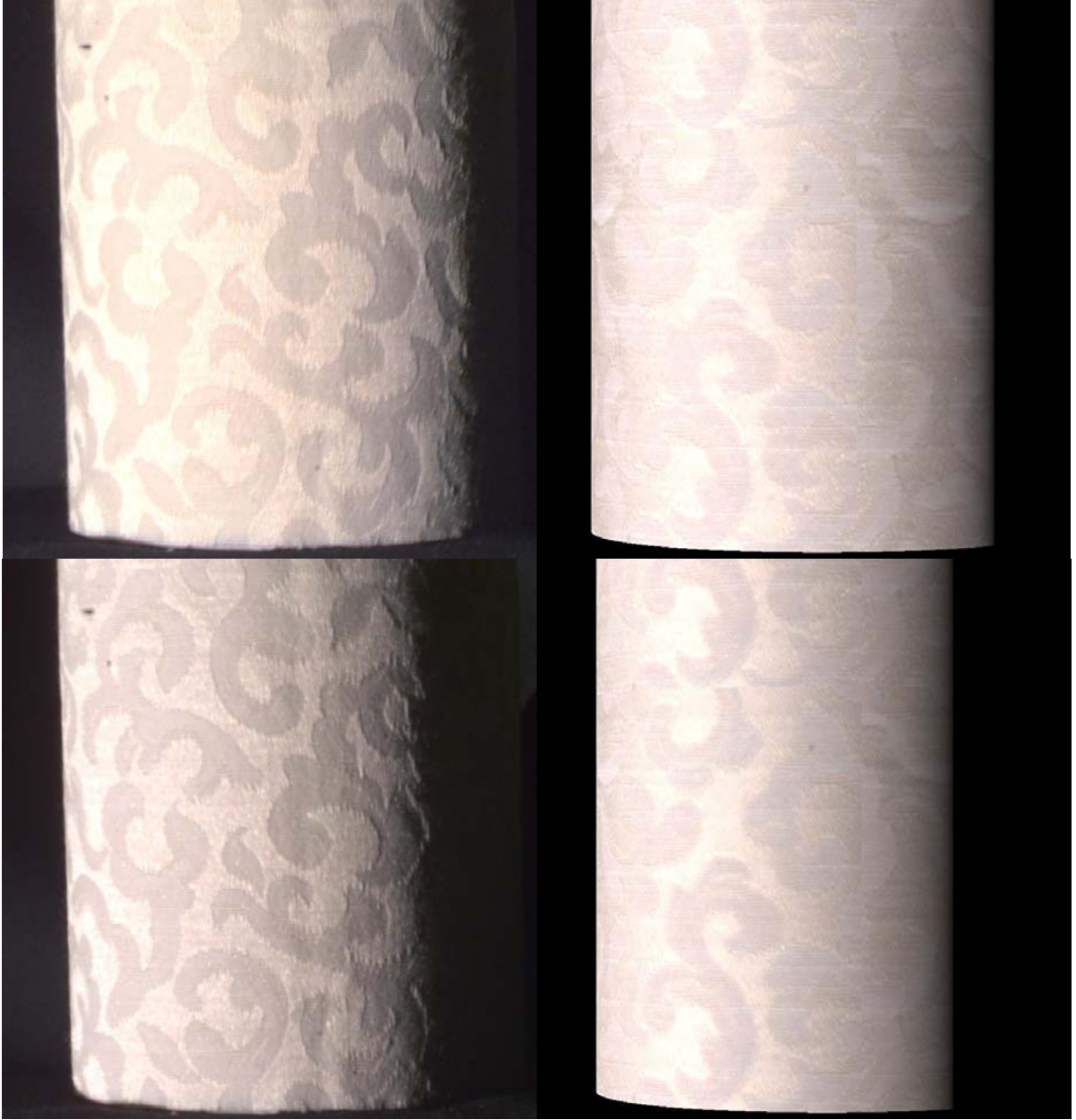
Figure 4.3: Left: Photographs of cylinder with white fabric. Right: Software rendered approximation of same scene geometry using measured SBRDF of white fabric. The top and bottom pairs differ only in light position.
