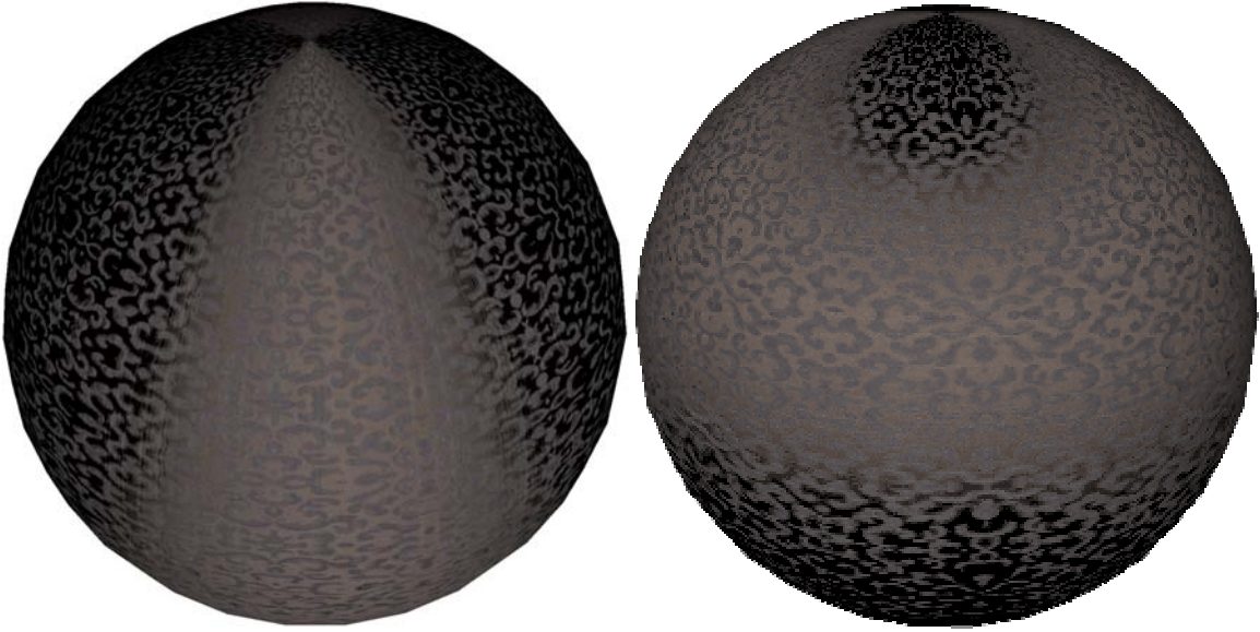
Figure 4.4: Specular component of anisotropic White Fabric sample. In the left image the silk background threads run horizontally, creating a cat's eye-shaped highlight. In the right image the background threads run vertically, creating a crescent-shaped highlight. The cotton foreground threads are less specular, but still anisotropic, creating a broad, elongated highlight.
