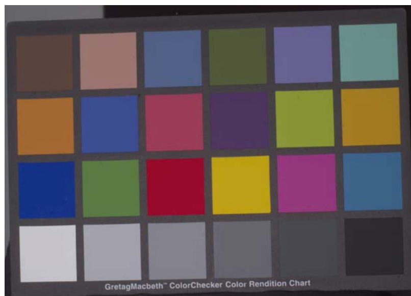
Figure 3.7: Macbeth ColorChecker chart photographed at high dynamic range and corrected for camera response.
