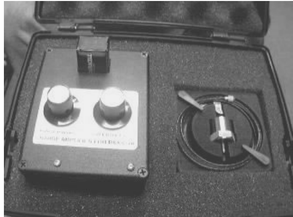
Figure 1: Kit consists of an accelerometer, a cable, a charge amplifier (shown with battery installed), and a carrying case.
