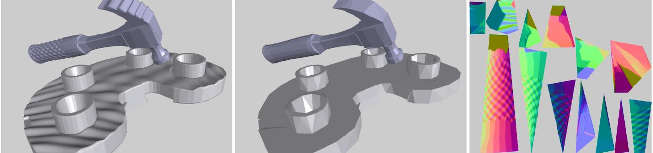
Figure 1: **Haptic Rendering of Interaction between Textured Objects.** From left to right: (a) high-resolution textured hammer (433K polygons) and CAD part (658K polygons), (b) low-resolution models (518 & 720 polygons), (c) hammer texture with fine geometric detail.
