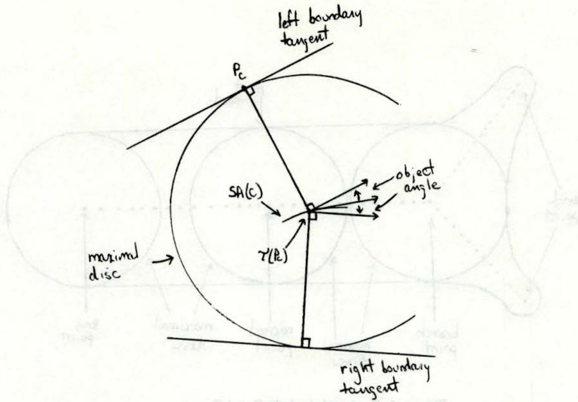
Figure 2: Normal Point Geometry (Point Contact)
