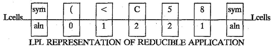
The representation of Figure 2.10 amounts to a record of a pre-order traversal of the parse tree of Figure 2.9, and can be easily generated from the FFP text in  $O(n)$  time and constant space by a pre-processor. This is the representation we choose to use in the FFP architecture. Its advantages include the use of fewer lcells than would be required by the more straightforward approach of using balanced constructor symbols.
