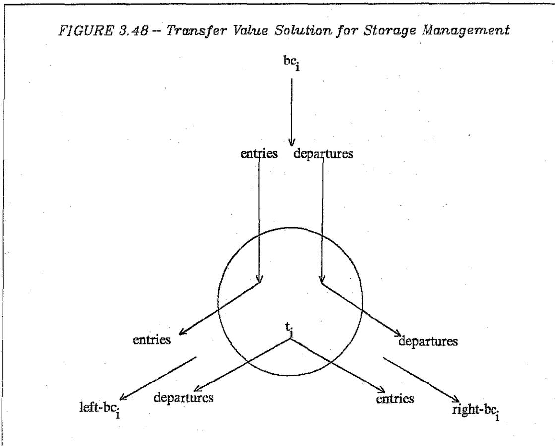
As shown in Figure 3.48, once  $t_i$ , a solution for storage management, is computed by the tcell at level  $i$ , it can send off *left\_bc* and *right\_bc* tuples to its left and right children as follows:
