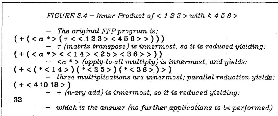
FFP reductions are completely local in nature and are tightly encapsulated with respect to the rest of the program. This fact allows immediate, completely parallel and non-interfering execution of all innermost applications (hereafter referred to as *reducible applications*, or *RAs*), and it is this property of FFP languages that makes them so attractive for multiprocessor support. User programs are actually written in FP, a human-engineered version of FFP
