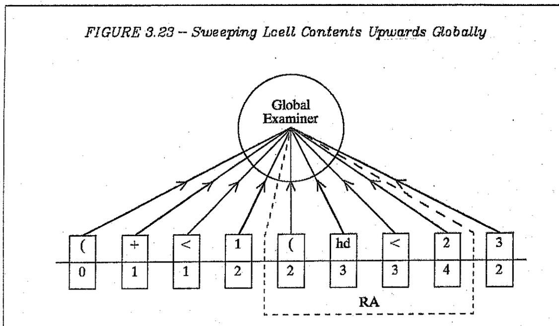
Of course, we need to accomplish the same thing using a binary tree-structure in place of the n-ary tree-structure of Figure 3.23. The n-ary tree method is easy to understand because one process with unlimited access to information is used within the single parent node. When using a binary tree structure, on the other hand, we must contend with a number of tcell processes, each of which has access only to the limited amount of information available from its two children.
