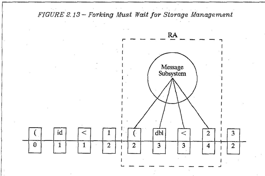
DOT supports the fork operation during a period of time called storage management, when all LPL programs are held in a quiescent state and execution contexts can be shifted about on the horizontal connections between lcells. A variety of mechanisms for the scheduling of this period are possible. Chapter 6,
