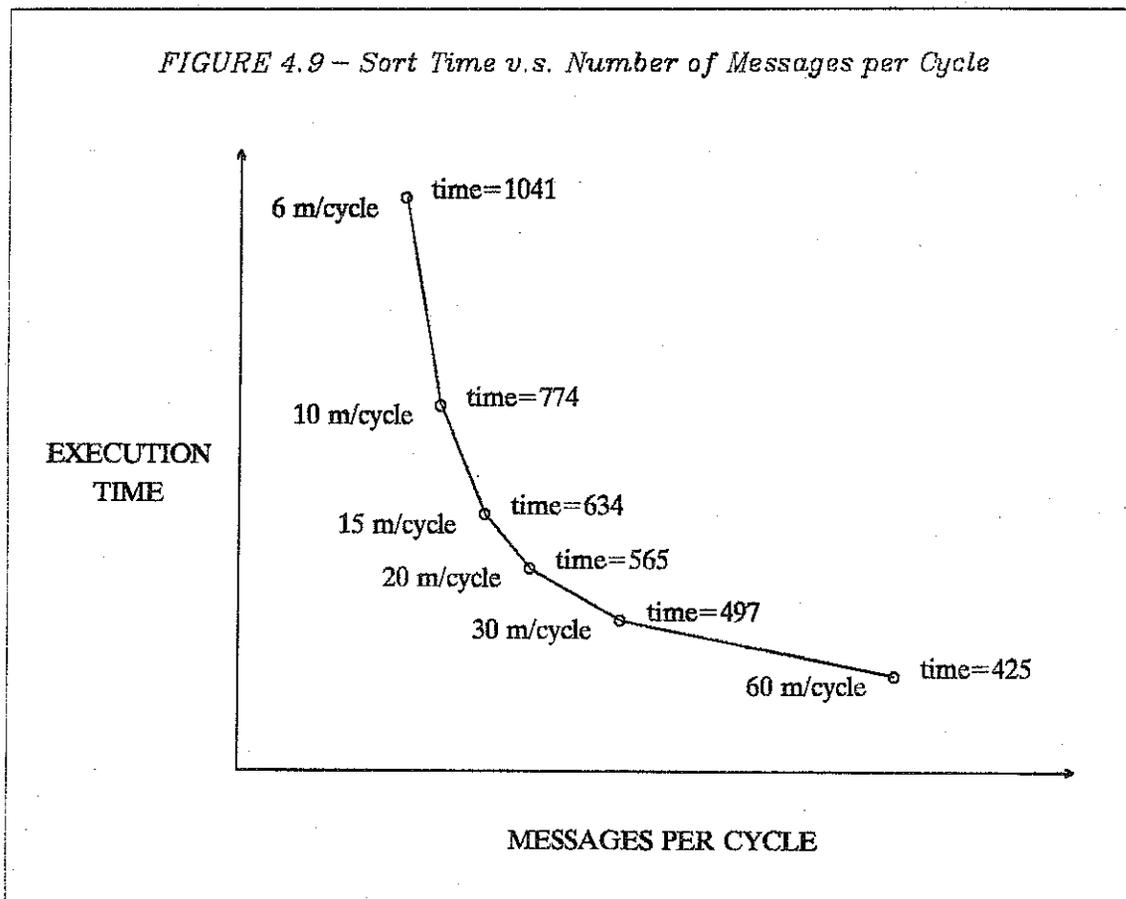
425, achieved by sending the 60 messages during one cycle, is quite close to the time of 497, achieved when two cycles are used (30 messages per cycle). The optimum execution time is approached asymptotically, so backing off and being "fair" to other programs in the machine is not as costly as might be expected.
