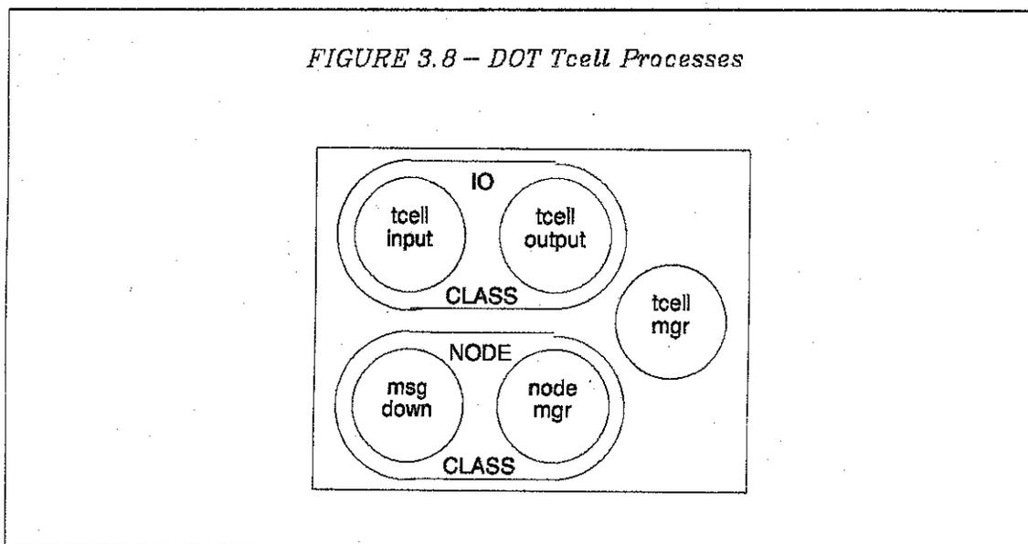
The rationale behind this choice of processes is provided by the process-oriented design methodology. Each tcell process performs duties that are best viewed separately from the others, and for which there is a simple sequential (cyclic) description.
