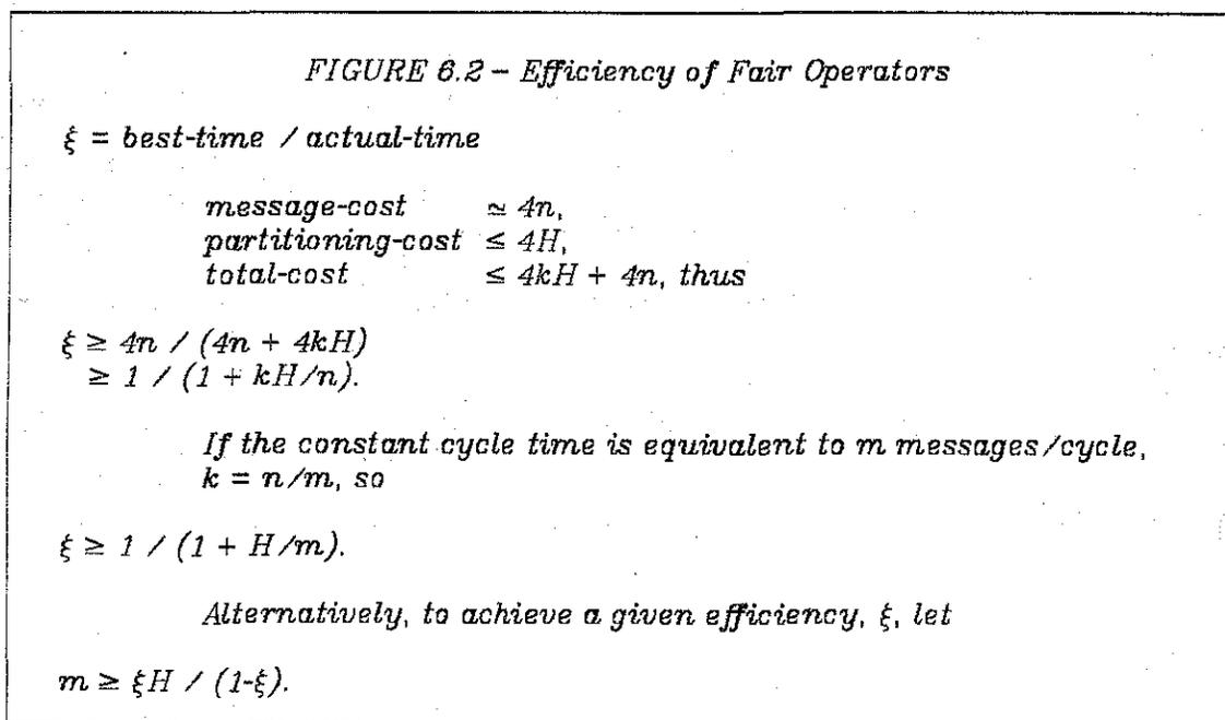
From the results of Figure 6.2, to achieve 50% efficiency in communication-bound RAs, the machine cycle should be set so at least  $H$  messages may be sent each cycle. For a machine of height  $H=20$ , to achieve 50% efficiency the duration of the execution phase should be at least  $(2H + 4H + 3) = 123\tau$ . If  $\tau$  is
