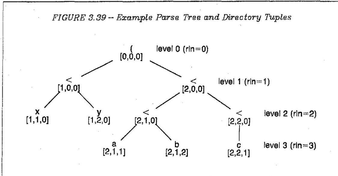
We now consider the tuple values that are passed in the upsweep and downsweep to compute the directories for the symbols of an RA. We make no assumptions here concerning the level of truncation. DOT presently provides LPL programs with a four-level directory, but the following algorithms work with truncation at any level. All examples will perform truncation at level 3, as in Figure 3.39.
