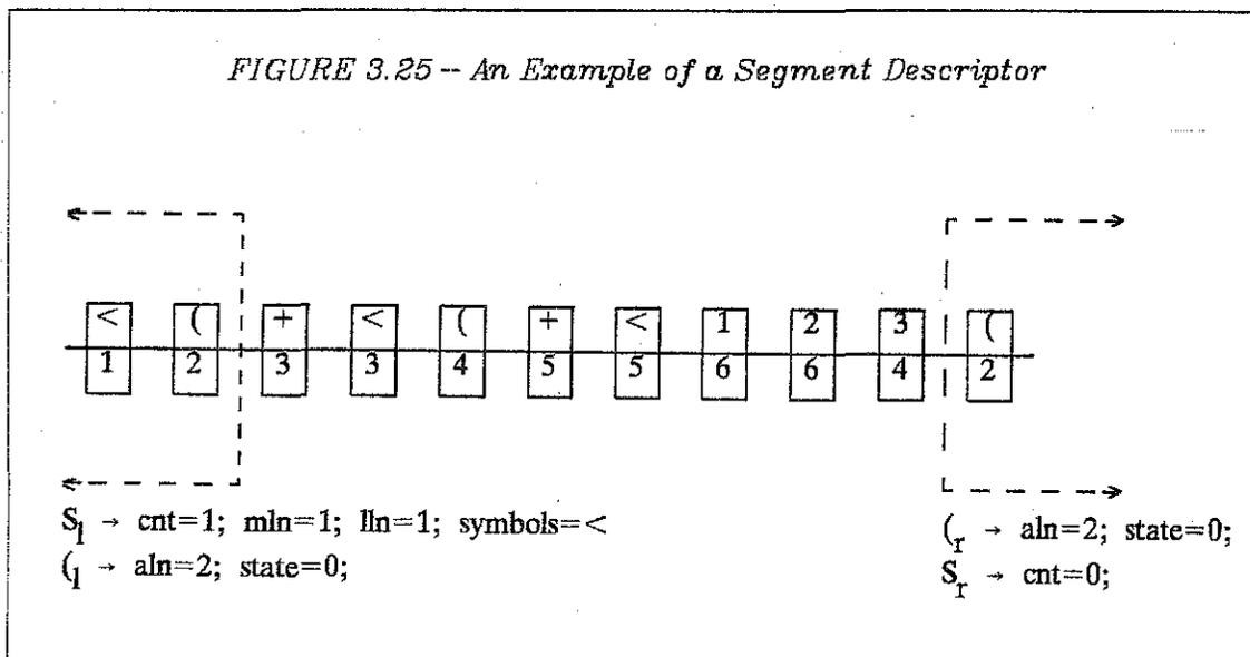
The example in Figure 3.25 shows that all the information required by neighboring application symbols on either side of the example segment is
