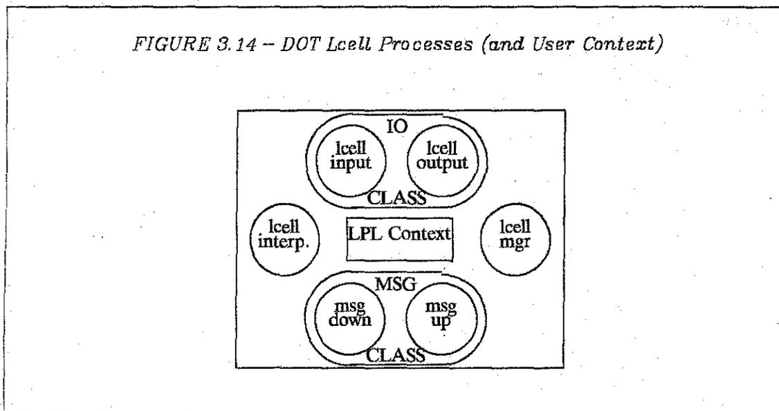
The `lcell_input` process is connected to the end of an io channel through which all LPL programs required by any RA in the machine arrive, and it filters this flow of information to select and load only the LPL code segment that is locally required (if any). Everything else is thrown away. As soon as the correct code segment is loaded, the input process starts the LPL interpreter by sending it a beginning code address. Figure 3.15 shows the lcell input process.
