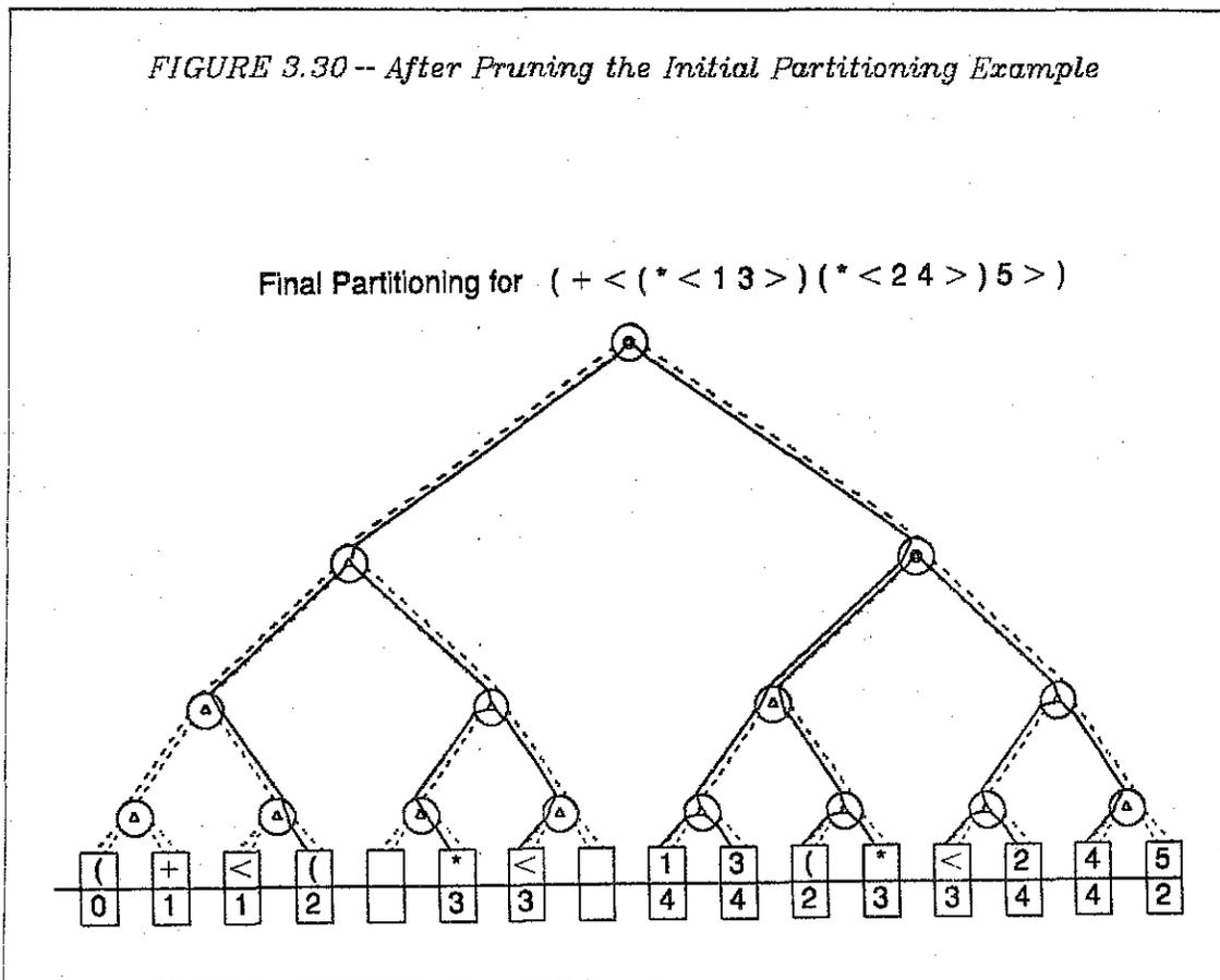
area channels re-routed appropriately. The final position of the two top of area nodes is shown by circling their nodes.
