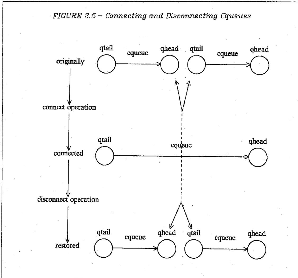
The ClassC entry templates for the `cqueue` `qhead` and `qtail` objects (which summarize the operations of which a cqueue is capable) are shown in Figure 3.6. The `connectw` operation connects two cqueues as discussed above, and delays the connecting process until an `eot_alert` (for end-of-transmission) is performed by a sending process on the cqueue `qtail`.
