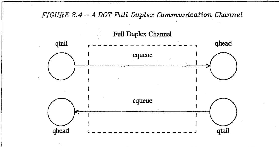
A cqueue has a variety of interesting properties. Most importantly, a cqueue implements a "safe" message transmission mechanism. Both sender and receiver are synchronized by a message transfer; a sender is delayed until a receiver requests data, and vice-versa. This corresponds to the synchronization that is necessary between hardware processes that operate from different clocks. DOT thus encapsulates concern for the synchronization that must be present in the realization at this level.
