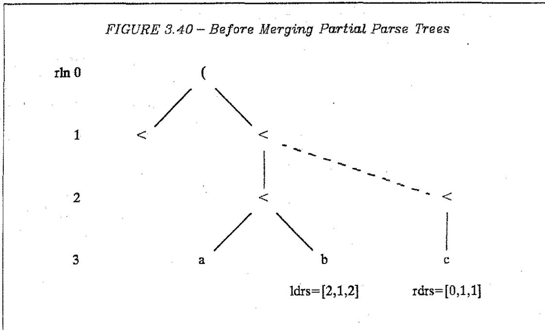
Note that the parse tree class implied by *ldrs* in Figure 3.40 does not include nodes for all the operator symbols of the actual RA. This is a result of the limited precision of *ldrs*, the relative directory of "b". Truncation effects are absent because no symbol of the RA is nested deeper than three levels.
