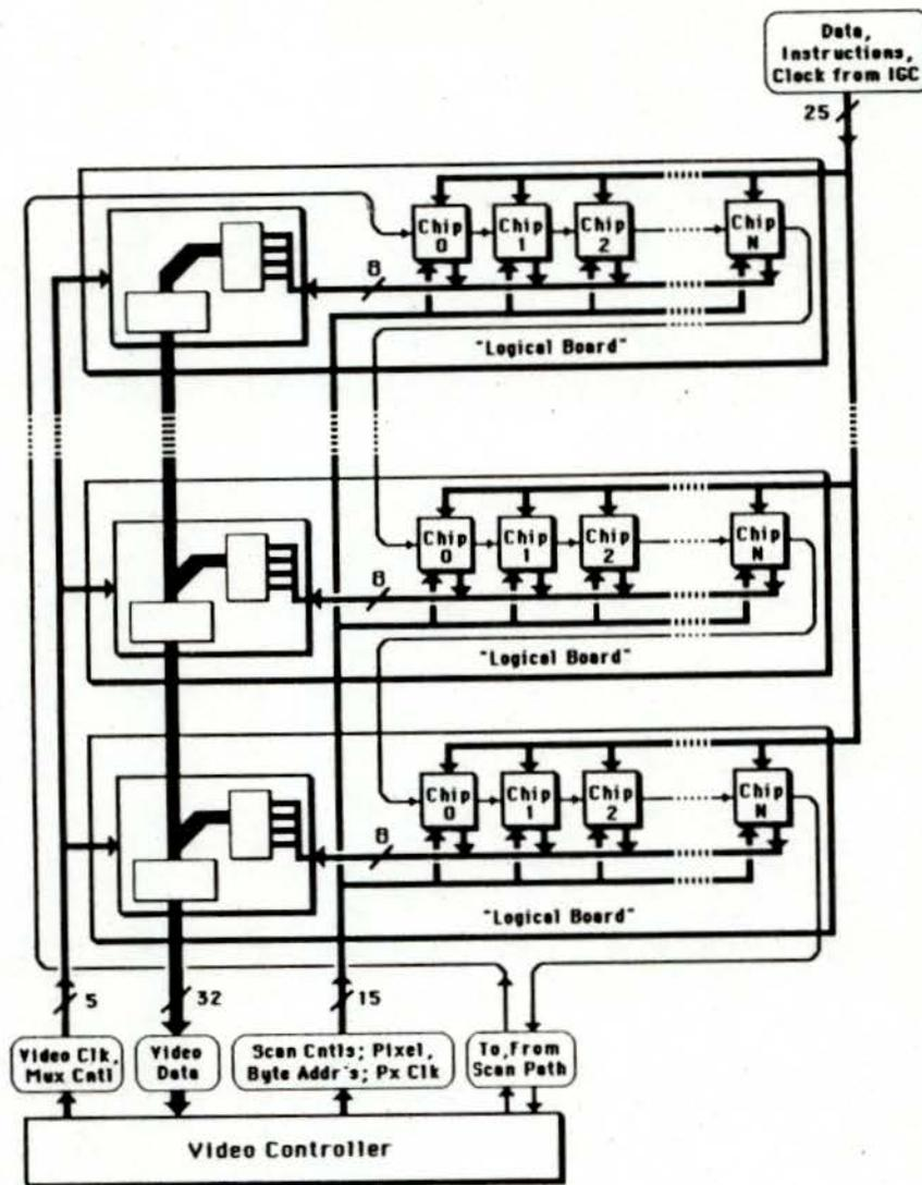
Figure 2: Pixel-Planes Smart Frame Buffer organization.
