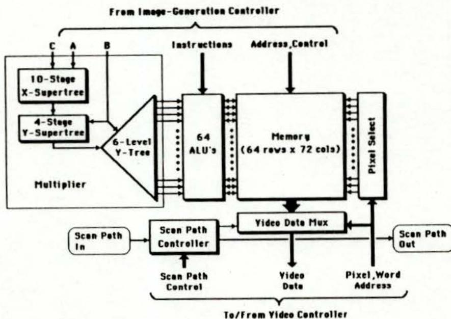
Figure 3: Block diagram of the Pixel-Planes memory chip.
