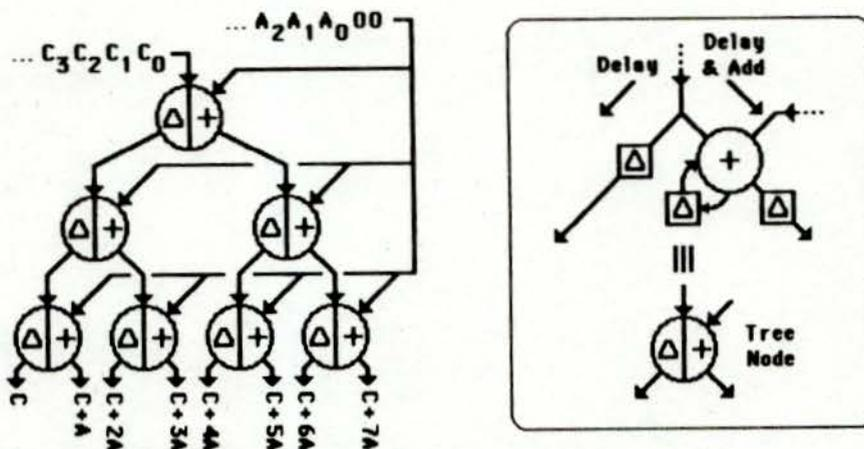
Figure 4: Conceptual model of binary-tree linear expression evaluator.
