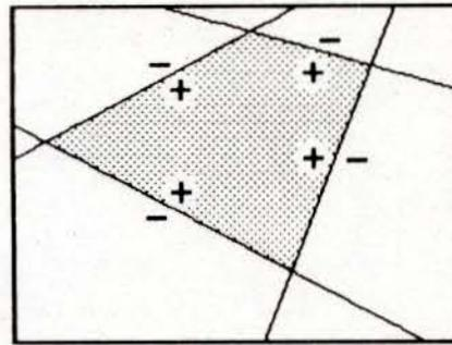
**Figure 10: Scan-covering polygons using linear expressions.**
