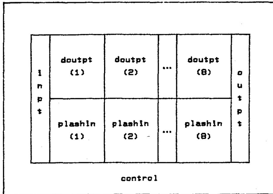
To execute this interconnection of eight 'plashin' shift register cells, I used 19 simple module processes. In addition to the 'plashin' module process, which was obtained by copying the specification (see Figure 3-6):
