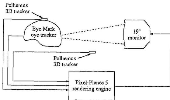
Figure 1: Hardware configuration
