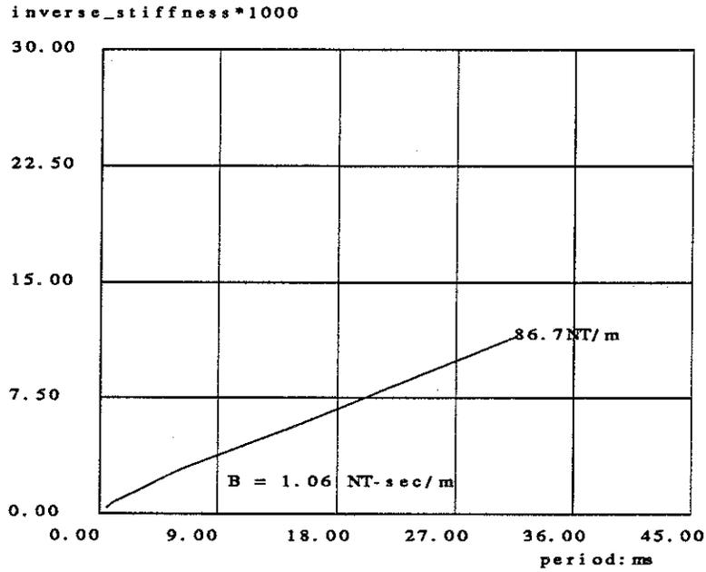
Figure 7.3: Joystick 1/stiffness (in m/N) versus sampling period (in ms).
