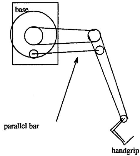
Figure A.2: The special elbow-bend joint with a parallel bar.
