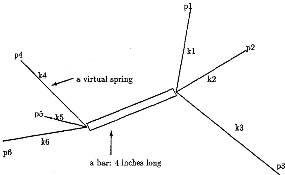
The goal is to find the zero-force position and orientation of the bar, where p1 to p6 are positions in 3-D, and k1 to k6 are the elastic constants for springs.
