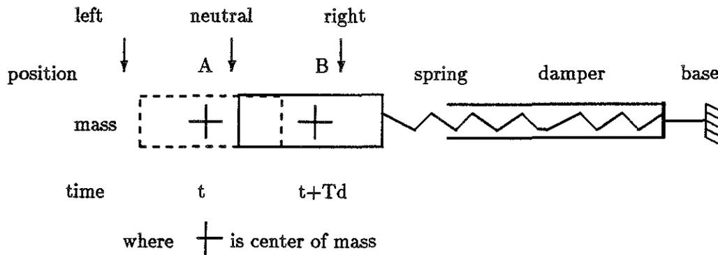
Figure 2.1: A spring and mass system in oscillation
