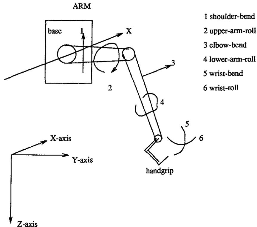
Figure A.1: The six ARM joints.
