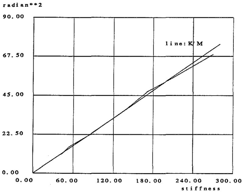
Figure 7.2: ARM's shoulder-rotation frequency squared (in radian) versus stiffness (N/m).
