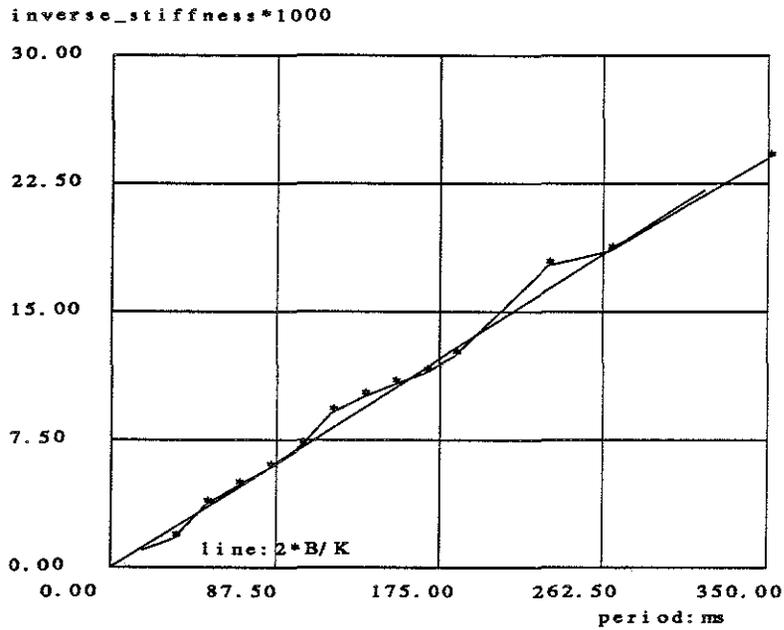
Figure 7.1: ARM's shoulder-rotation 1/stiffness (in m/N) versus sampling period (in ms).
