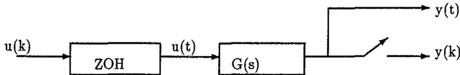
Figure 6.4: A digital model based on sample and hold, where ZOH is a zero-order-hold (sample-and-hold),  $u(k)$  is discrete input data,  $y(k)$  is discrete output data,  $u(t)$  is an analog input signal after sample-and-hold, and  $y(t)$  is the analog output signal.
