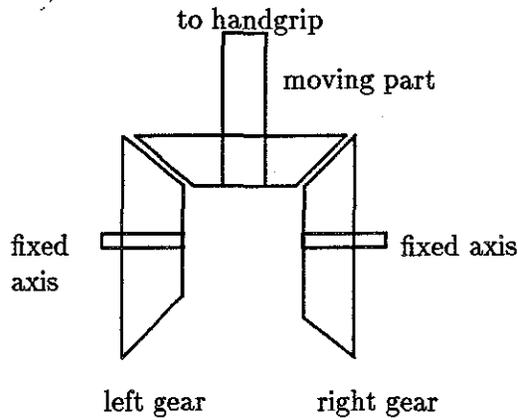
Figure 10.1: Differential gears at the ARM wrist joint.
