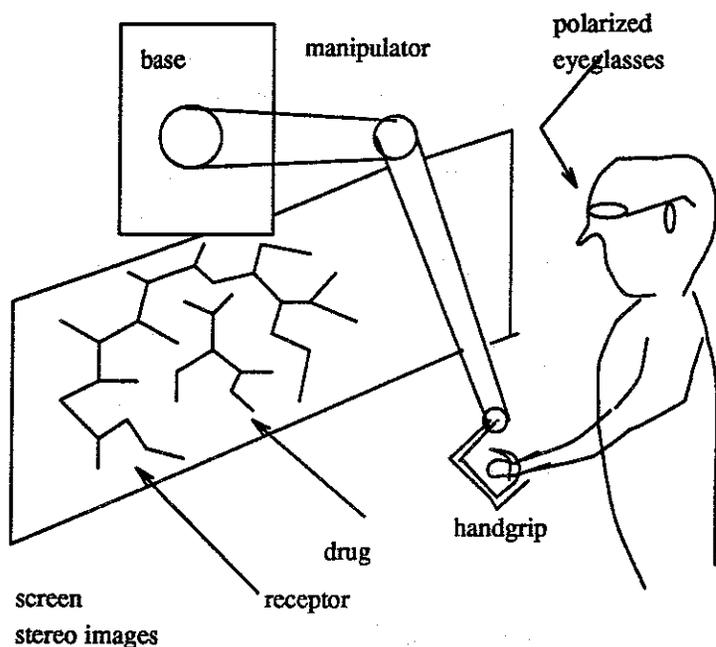
The molecular scientist is using the system to dock the drug into the receptor. The system has visual and force display at the same time.
