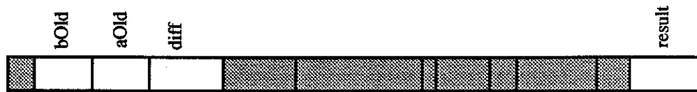
Figure 3-13. Fourphront scavenges bits from the memory-transfer area and from the texture area of the default usage. These bits are used to compute the fixed-width intersection curve.
