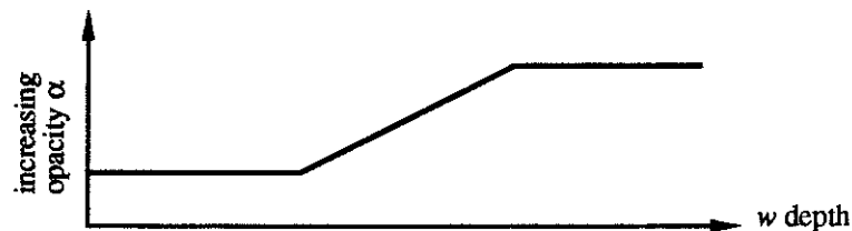
Figure 2-10. Opacity can be used as a depth cue in the w -direction without significantly interfering with the usual depth cues in the z -direction. For example, points on the surface near the eye are rendered nearly transparent, while points far away in w are nearly opaque. Fourphront uses a linear opacity ramp that is clamped at controllable near and far values.
