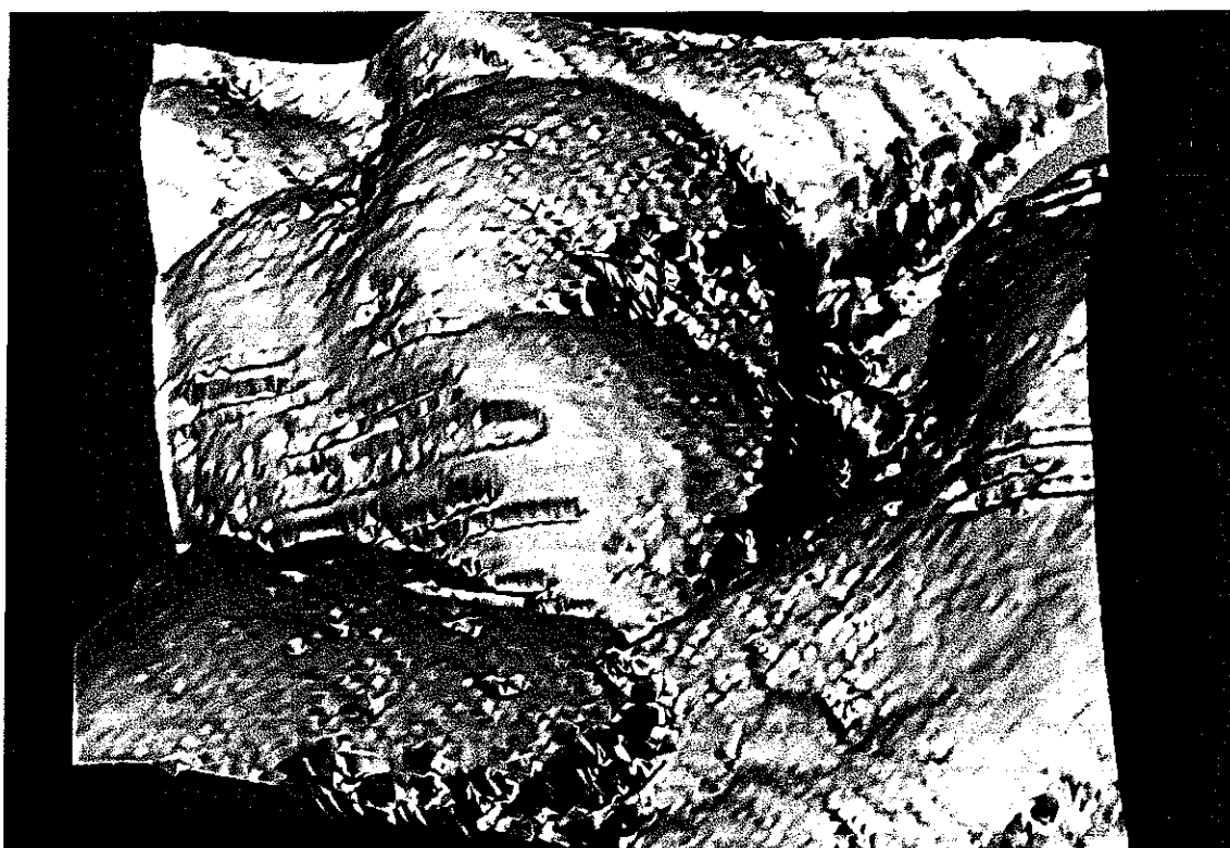
Figure 3.1 Graphite planes. This is a rendered image of an ion-bombarded highly-oriented pyrolytic graphite (HOPG) sample. The large scrapes in the center are visible even on a gray-scale image; the more subtle diagonal striping in the upper right corner is accentuated by highlighting and indicates graphite sheets that have pushed up out of the surface.
