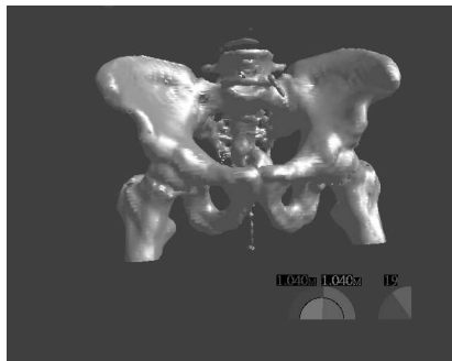
Figure 5. - same study as Figure 3. Bone surface (49552 triangles) generated in 409 msec. View update rate 19 fps
