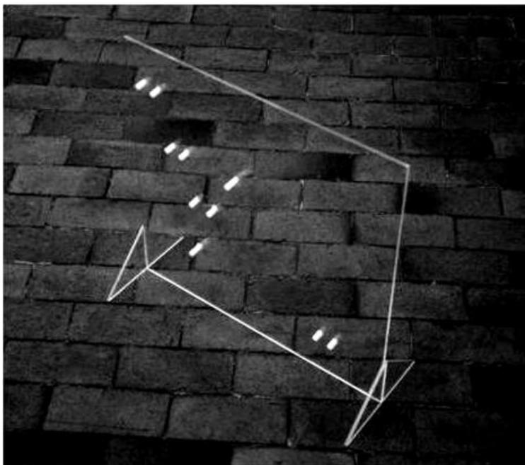
**Figure 3.7:** Photograph of the tracking arm calibration jig made of transparent Plexiglas. (The photo is taken on the brick floor.) Several pockets made of pairs of pegs were used to calibrate translation and rotation of the mechanical tracking arm.
