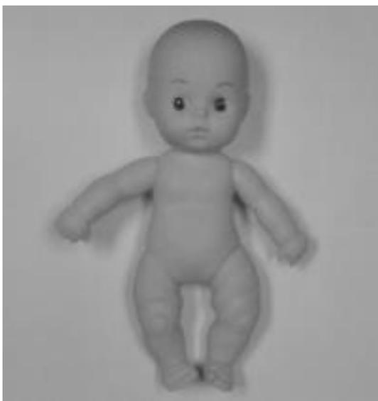
**Figure 3.39.a:** Photograph of the doll phantom, whose height is 17.5cm. This phantom is placed in a water tank and scanned by ATL Mark-4 echography scanner with 3.5 MHz linear scanhead.
