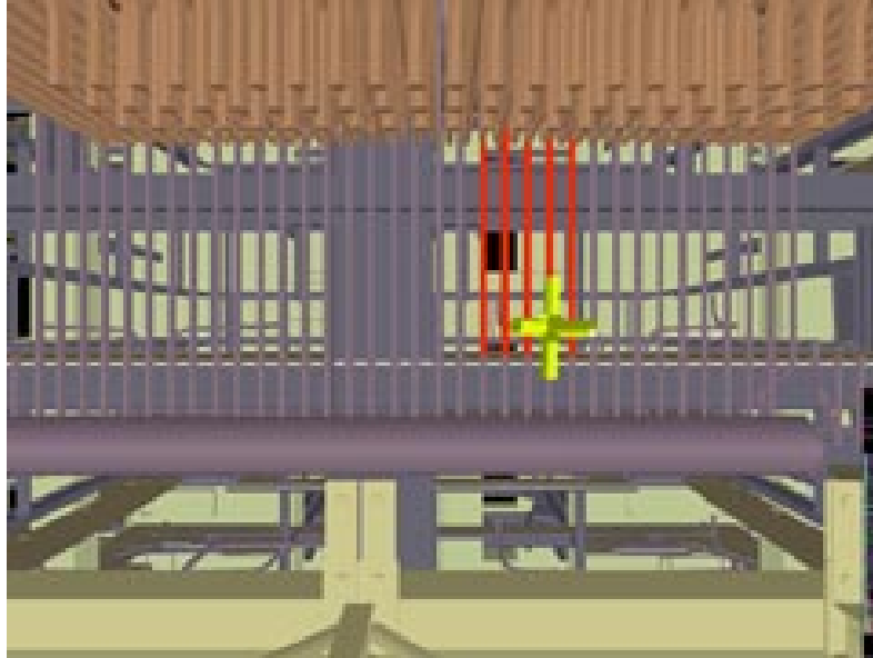
Figure 9: Interactive collision detection between a moving objects and pipes in the powerplant.
