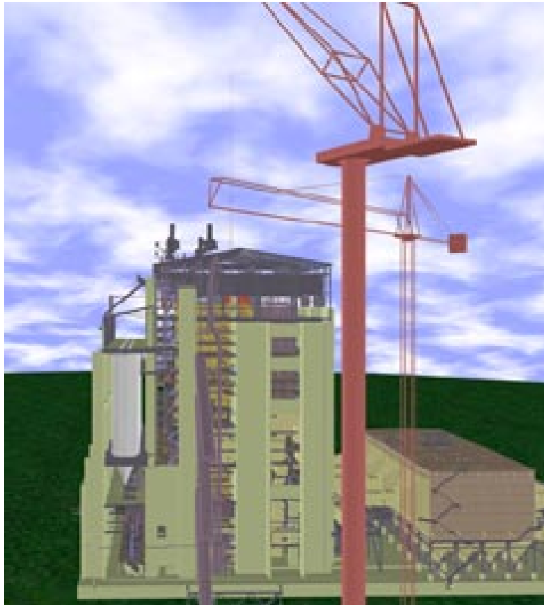
Figure 7: CAD model of a coal-fired powerplant with more than 15 million triangles. The model consists of more than 1800 objects and takes more than 1.3GB on disk.
