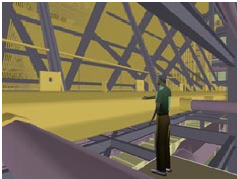
Figure 8: Proximity queries between an avatar and the powerplant model. IMMPACT takes a few milliseconds to perform these queries.
