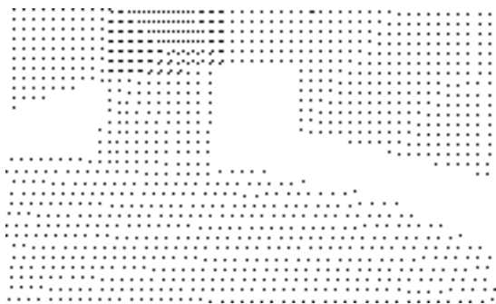
Figure 4.1: When pixels are transformed from the reference image to the destination image, the transformed locations do not form a regular grid in the destination image. Instead, they are irregularly located. This figure shows the destination-image locations of transformed pixel centers for a portion of a frame from the kitchen walkthrough. Only one (of two) reference frame's transformed pixel centers are shown.
