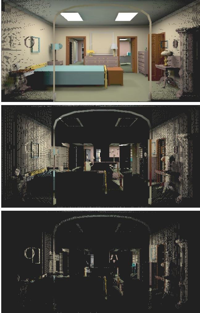
Figure 4-5. Layers of a LDI. The images show, from top to bottom, the samples at depth 0, 1 and 2 of a LDI. The side walls are present in more than one layer not because of visibility, but rather because they are not adequately sampled by the central view; when the LDI is warped to a view where better sampling is necessary, the successive layers will unfold, ensuring better reconstruction.
