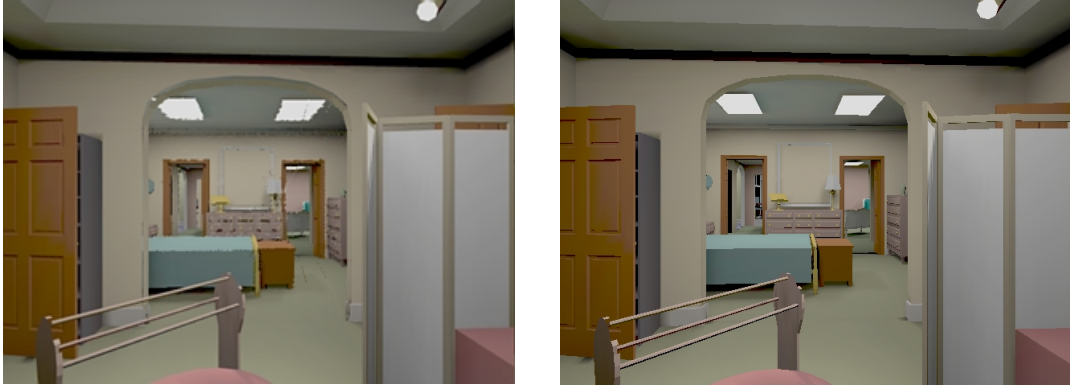
Figure 4-3. Example Layered Depth-Image. The doorway of the left snapshot is rendered as a layered depth-image. Notice the absence of the “tears” of Figure 4-2. For comparison, the right snapshot is rendered with conventional geometry.
