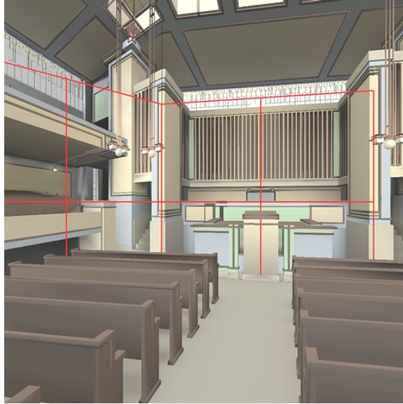
Figure 5-10. Images and Warped Geometry in the Church Model. We show two images (outlined in red) surrounded by warped geometry. This frame is rendered from an eye location far behind the image-sampling viewpoint. The geometric distortion, particularly in the ceiling, is very noticeable. Nevertheless, there are no discontinuities at the geometry-image border.
