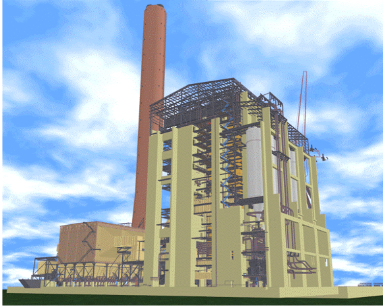
Figure 1-3. Coal-fired Power Plant. This is a very large model (over 13 million triangles) of a coal-fired power plant. The main building is over 250 feet high (50 levels) and contains large arrays of piping, generators, and other machinery. Courtesy of ABB Engineering.
