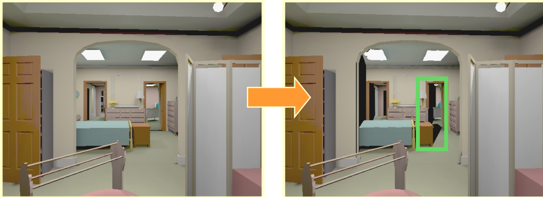
Figure 4-2. Limitation of Single-Image Warping. If we move in three-dimensional space, regions previously occluded become visible. A single reference image cannot capture the additional visibility data. In both snapshots, the scene visible through the central doorway is rendered as a warped image (the rest is rendered using conventional geometry). The left snapshot is the view from the image-sampling viewpoint. In the right snapshot, we have slightly translated our viewpoint. Notice the “tears” or sharp shadows that have appeared because we do not have pixel samples for the previously occluded surfaces (note: we have outlined the tear to the right of the bed).
