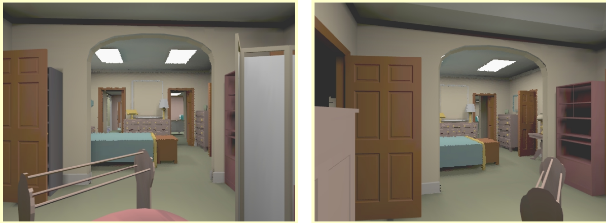
Figure 1-6. Image Warping. The view through the doorway is rendered as an image. In the right snapshot, we have translated and rotated the viewpoint to one side. Per-pixel depth values are used to “warp” the image to the new viewpoint. We employ a layered depth image to store information for surfaces visible in the right snapshot that are not visible in the original snapshot.
