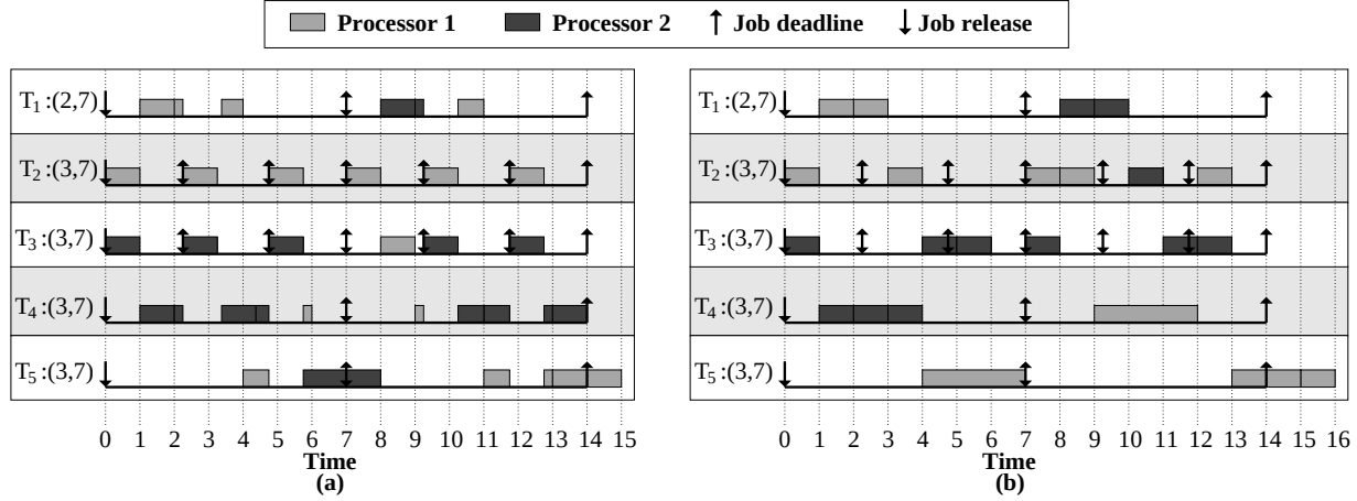
Figure 1.5: Two-processor (a) GEDF and (b) NP-GEDF schedules.
