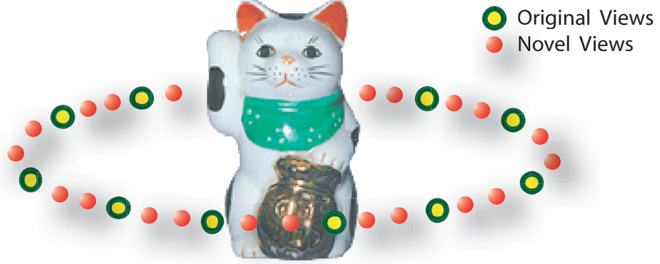
Figure A.1: Typical eigen-texture method captures images along a circular path around an object. Synthesis of novel views is only possible along this path.
