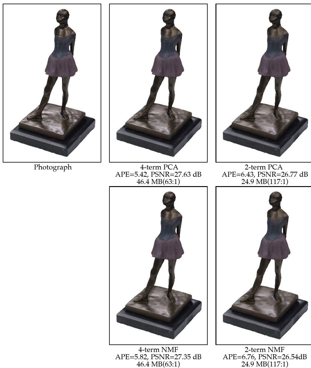
Figure C.3: Comparison between PCA and NMF approximation methods. Using the same number of terms, PCA light field maps produce less error, but are slower to render than NMF.
