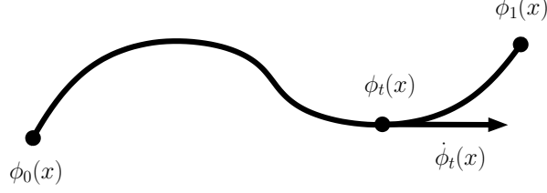
Figure 2.1: Velocity integration. The diffeomorphism \phi \in \text{Diff}_V(\Omega) evolves in time as a flow \phi_t . This flow is governed by the time-varying velocity field v_t . This process is demonstrated for a single point x \in \Omega .
