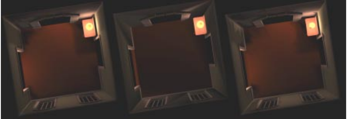
Figure 1.6: The benefits of handling surface attributes. On the left is an overhead view of the original radiositized Chamber model consisting of 10,423 polygons. In the middle is the result of simplifying the model while ignoring surface attributes. On the right, we use surface attributes to guide the simplification process, retaining more of the color information of the model. Each simplified model consists of 5,120 polygons.
