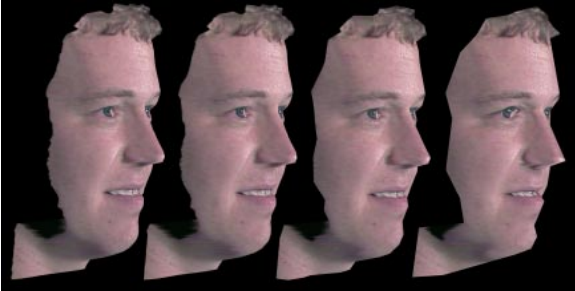
Figure 3.16: The original texture-mapped Head object and its LODs created by GAPS. From left to right these objects consist of 9,580 faces, 2,395 faces, 597 faces, and 148 faces.
