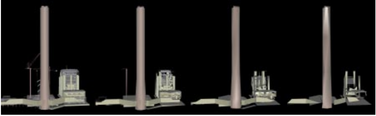
Figure 4.34: LODs created for the Power Plant model using GAPS. They consist of 12,731,154 faces, 9,558 faces, 2,405 faces, and 612 faces.
