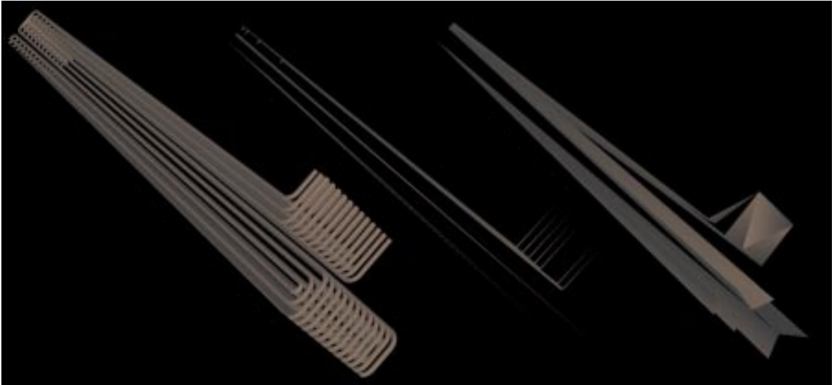
Figure 1.10: On the left is the original series of pipes consisting of 23,556 polygons that come from a power plant model. In the middle is the simplified output of an algorithm that does not merge unconnected regions of the model. On the right, GAPS merges unconnected regions of the pipes to produce a higher quality drastic simplification. Both approximations consist of roughly 90 polygons.
