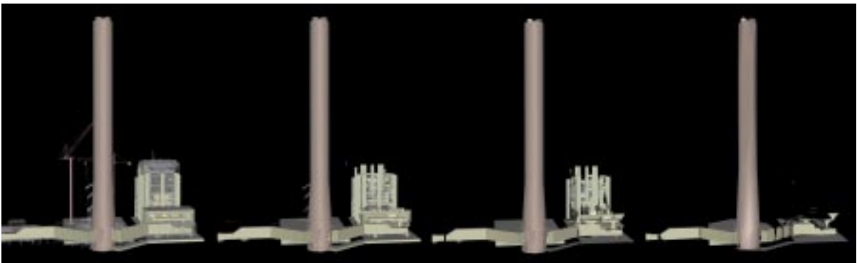
Figure 4.33: LODs created for the Power Plant model using the error quadric metric alone. They consist of 12,731,154 faces (the original model), 9,627 faces, 2,494 faces, and 607 faces.
