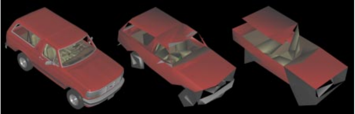
Figure 5.15: The original Bronco model consisting of 74,308 polygons and two HLODs consisting of 580 and 143 polygons respectively.
