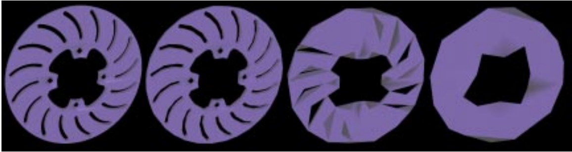
Figure 3.14: The original Rotor object and its LODs created by GAPS. From left to right these LODs consist of 4,736 faces, 1,184 faces, 296 faces, and 72 faces.
