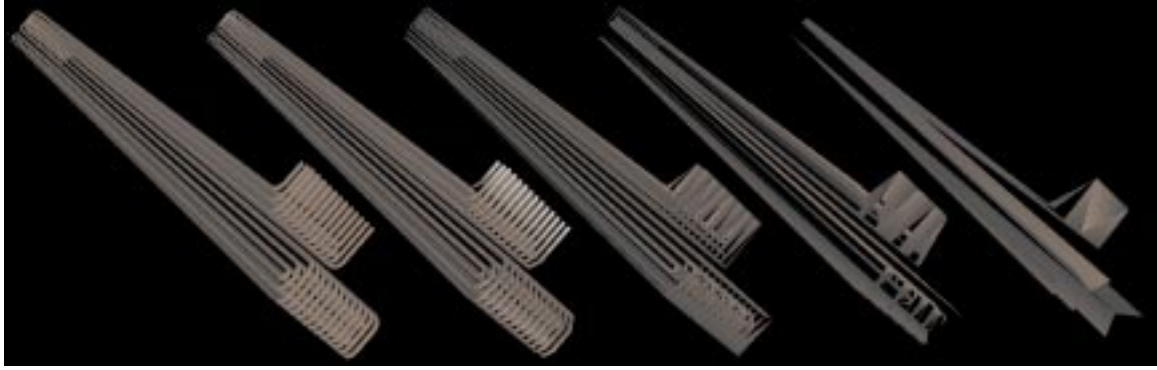
Figure 3.23: LODs for the Econ object created by GAPS using an adaptive distance threshold and surface area preservation. The pipes join together at the latter stages of simplification, preserving more of the surface area of the object as compared to Figure 3.22. From left to right these LODs consist of 23,556 faces (the original object), 5,888 faces, 1,470 faces, 368 faces, and 90 faces.
