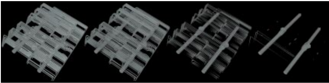
Figure 3.27: LODs for the ShDivWest object created by GAPS with no distance threshold and no surface area preservation. From left to right these LODs consist of 141,180 faces (the original object), 17,646 faces, 2,204 faces, and 272 faces.
