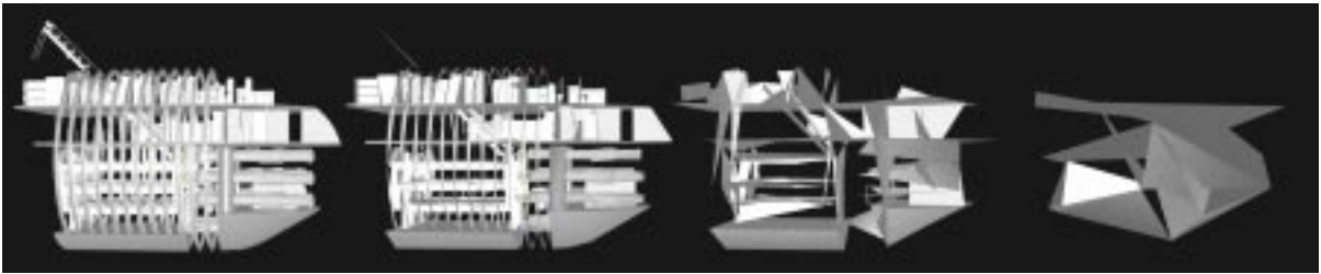
Figure 4.32: LODs and HLODs created for the Torpedo Room model using GAPS. They consist of 883,537 faces, 6,160 faces, 822 faces, and 95 faces.
