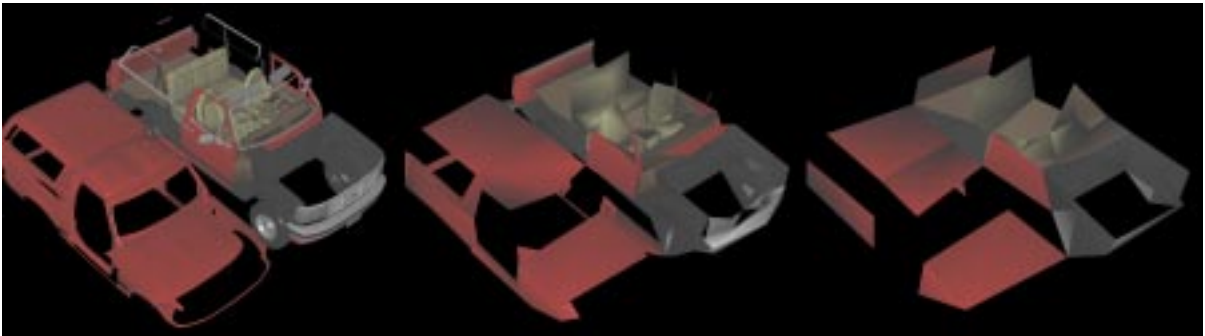
Figure 5.16: Dynamic modification of the Bronco model. We have moved the top of the Bronco in order to look into its interior. The two HLODs consist of 552 and 136 polygons respectively and took 3 seconds to recompute using 4 simplification processes on an SGI Reality Monster with 300 MHz R12000 processors and 16GB of main memory.
