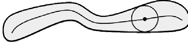
Fig. 2.1. The medial axis of a simple 2D object along with an inscribed maximal disk centered on the medial axis and tangent to the object boundary at two involute locations.
