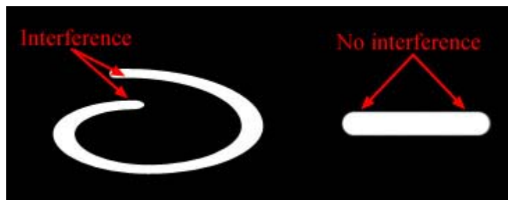
Fig. 7.18. Diagrams showing slices through two different slab-like objects. When dealing with tortuous objects, such as the one on the left, object edges may interfere during core computation if they are close to each other and if the image is noisy. This is not a problem with straighter objects, such as the one on the right.
