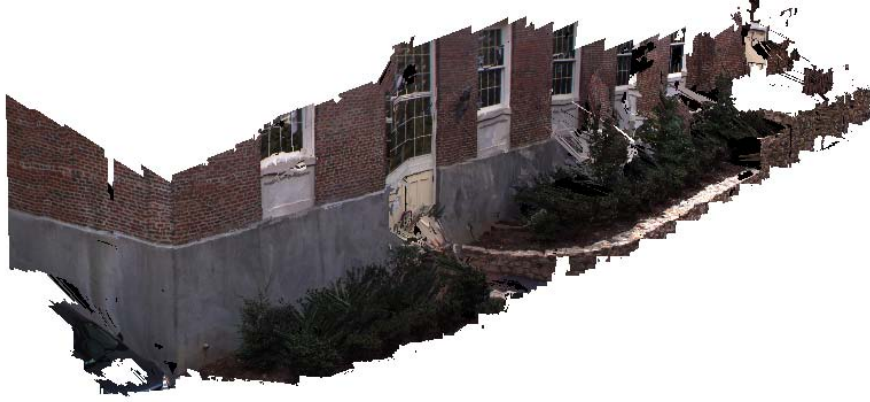
Figure 4.9: The reconstruction produced by our algorithm from several hundred frames of video. By testing only plane hypotheses with high prior probability, the reconstruction was achieved with only 48 plane hypotheses per frame at a speed of 50.0 Hz.
