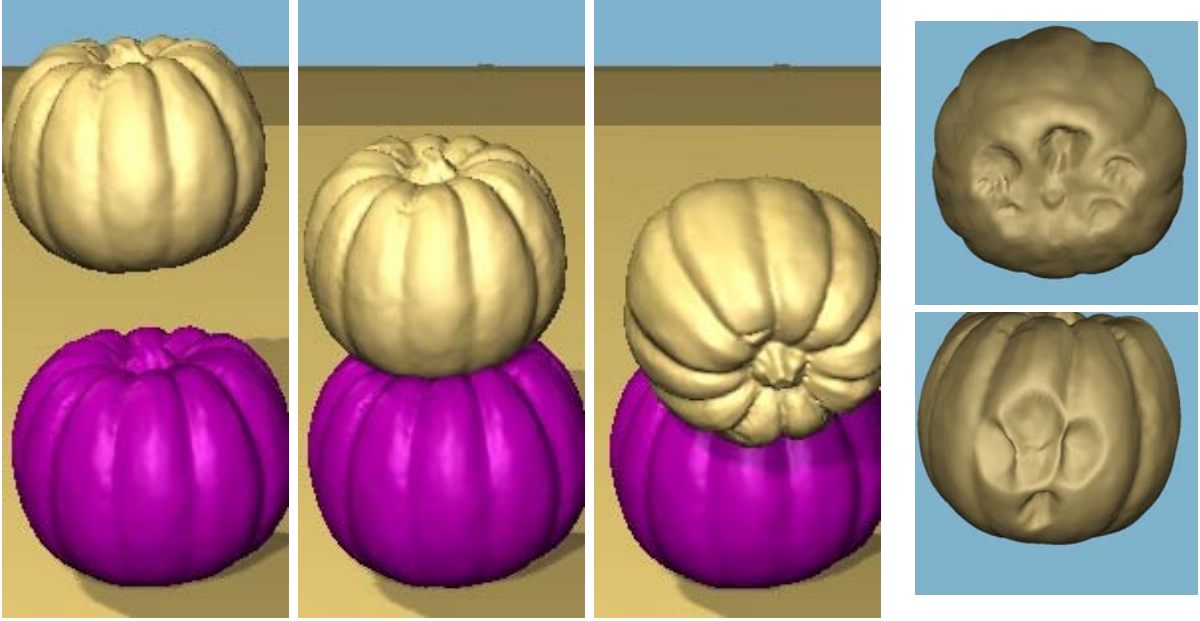
Figure 3.14: Deformations of High-Resolution Geometry. Left: Two deformable pumpkins are dropped on top of each other. Right: Detail view of the rich deformations produced on the top pumpkin during contact.
