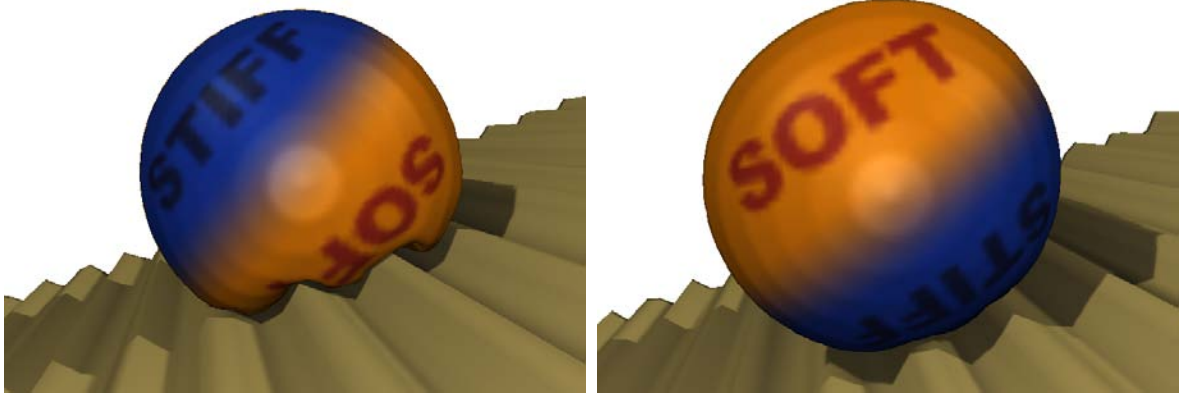
Figure 3.2: Simulation of Heterogeneous Materials. Efficient decoupled implicit integration enables fast simulation of a heterogeneous cylinder. Notice the large indentations and the resulting large contact area when the soft side collides with the ridged plane.
