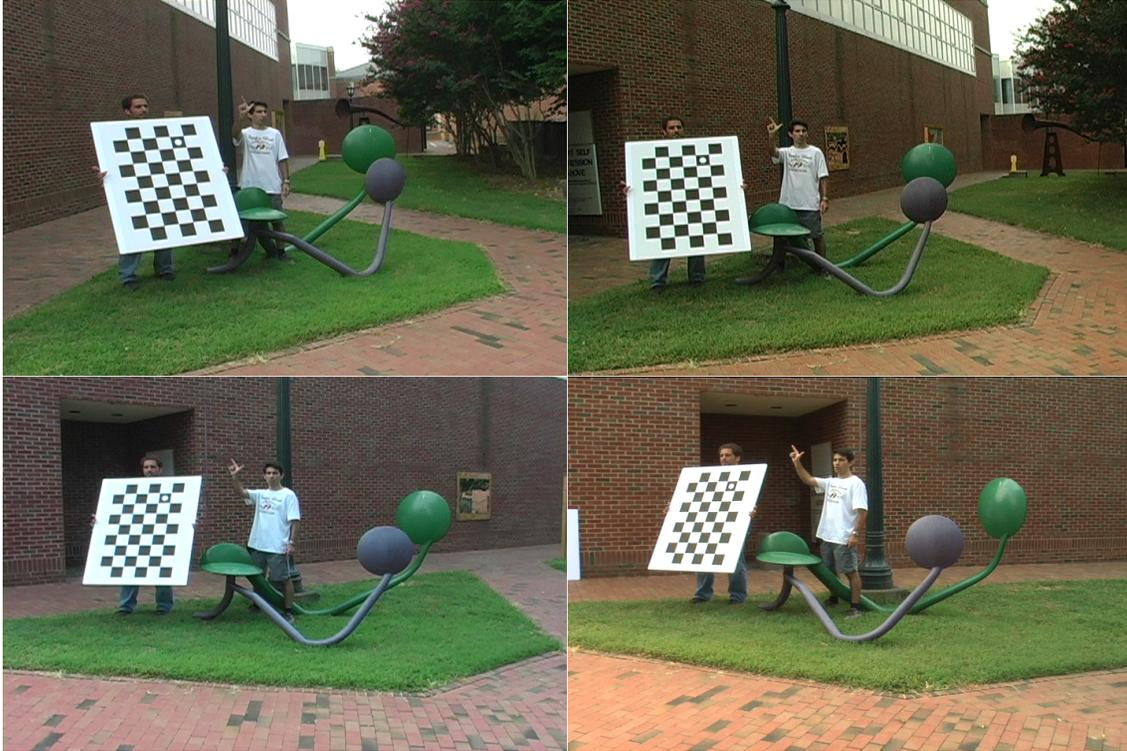
Figure 2.1: Camera network calibration session of the SCULPTURE outdoor datasets. This is one pose of the checkerboard calibration target. Four of the eight synchronized camera views are shown.
