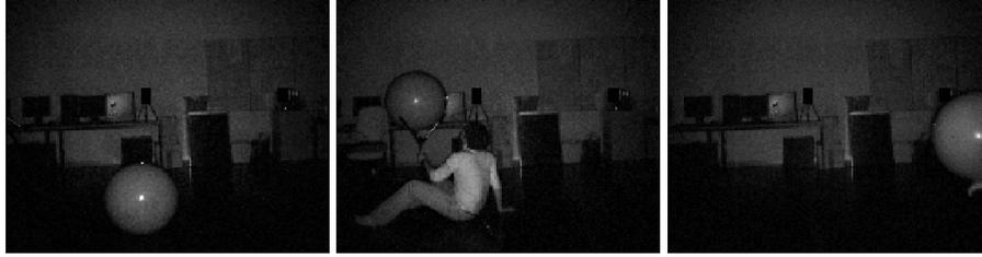
Figure 6.6: ToF camera Swiss Ranger 3100 intensity image sphere center highlights. To detect the highlight robustly and automatically, a simple Region of Interest (ROI) tracking method is applied.
