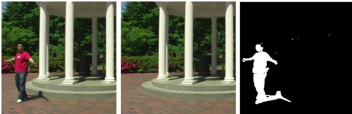
Figure 2.7: The silhouette from background subtraction. Left: an outdoor scene with a person; Middle: the trained mean background; Right: the silhouette(white) by thresholding the per-pixel background probability computed from Eq. 2.4. The shadow is labeled as a part of the silhouette.
