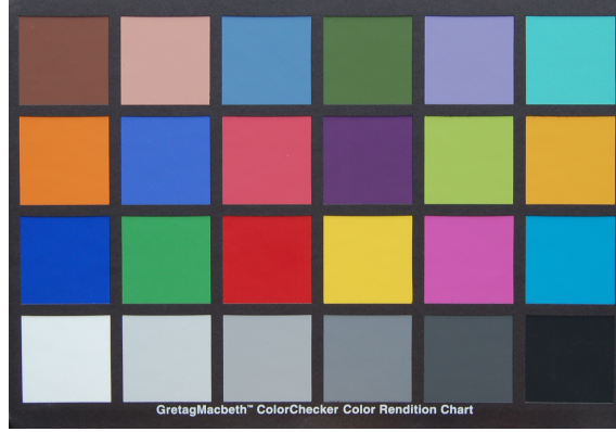
Figure 2.6: Macbeth color chart with 24 color patches with known reflectance.
