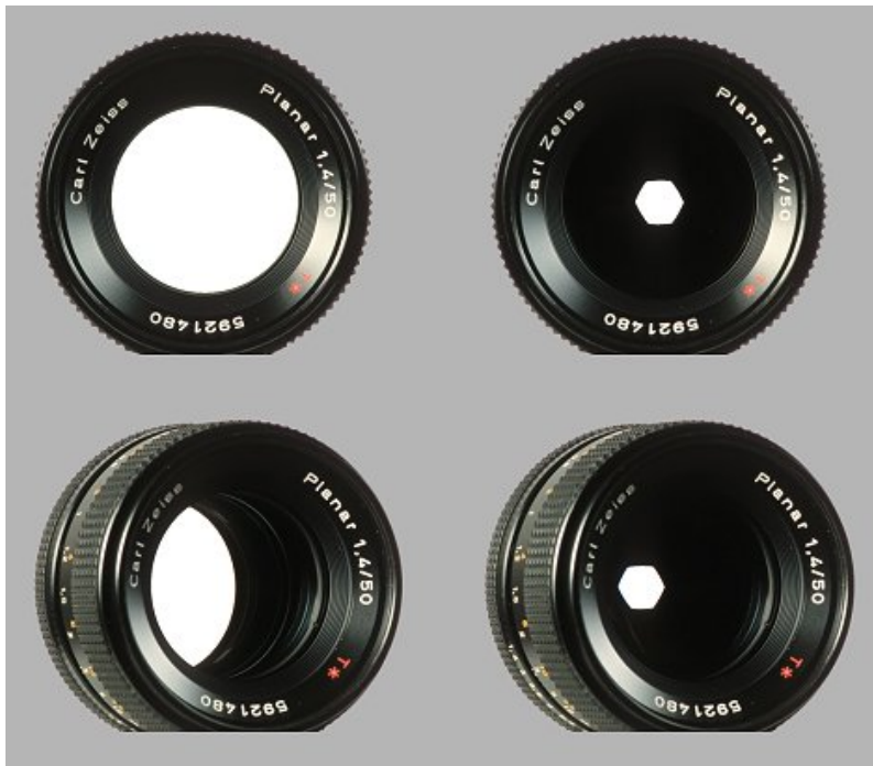
Figure 2.2: Vignetting Effect. (Top) Image taken with (left) a large aperture ( f/1.4 ) and (right) a small aperture ( f/5.6 ). (Bottom) Lens Images : (left) f/1.4 and (right) f/5.6 . ©Paul van Walree ( www.vanwalree.com )
