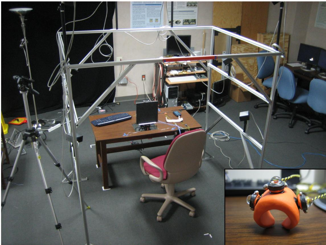
Figure 5.2: System constructed for space-warping studies. Inset shows the finger tracking ring.
