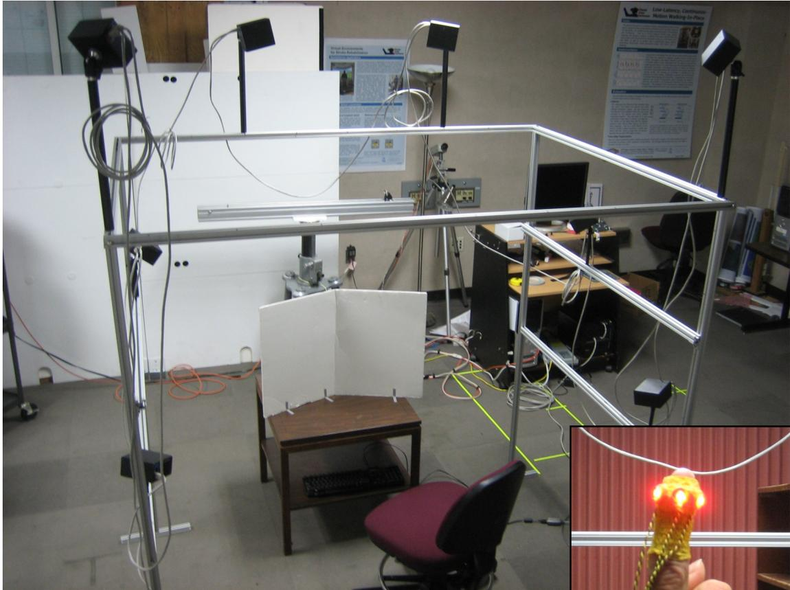
Figure 4.7: PhaseSpace® IMPULSE™ tracking cameras mounted on an aluminum frame. Inset shows tracking LEDs mounted onto an index finger using a self-adhesive athletic bandage.
