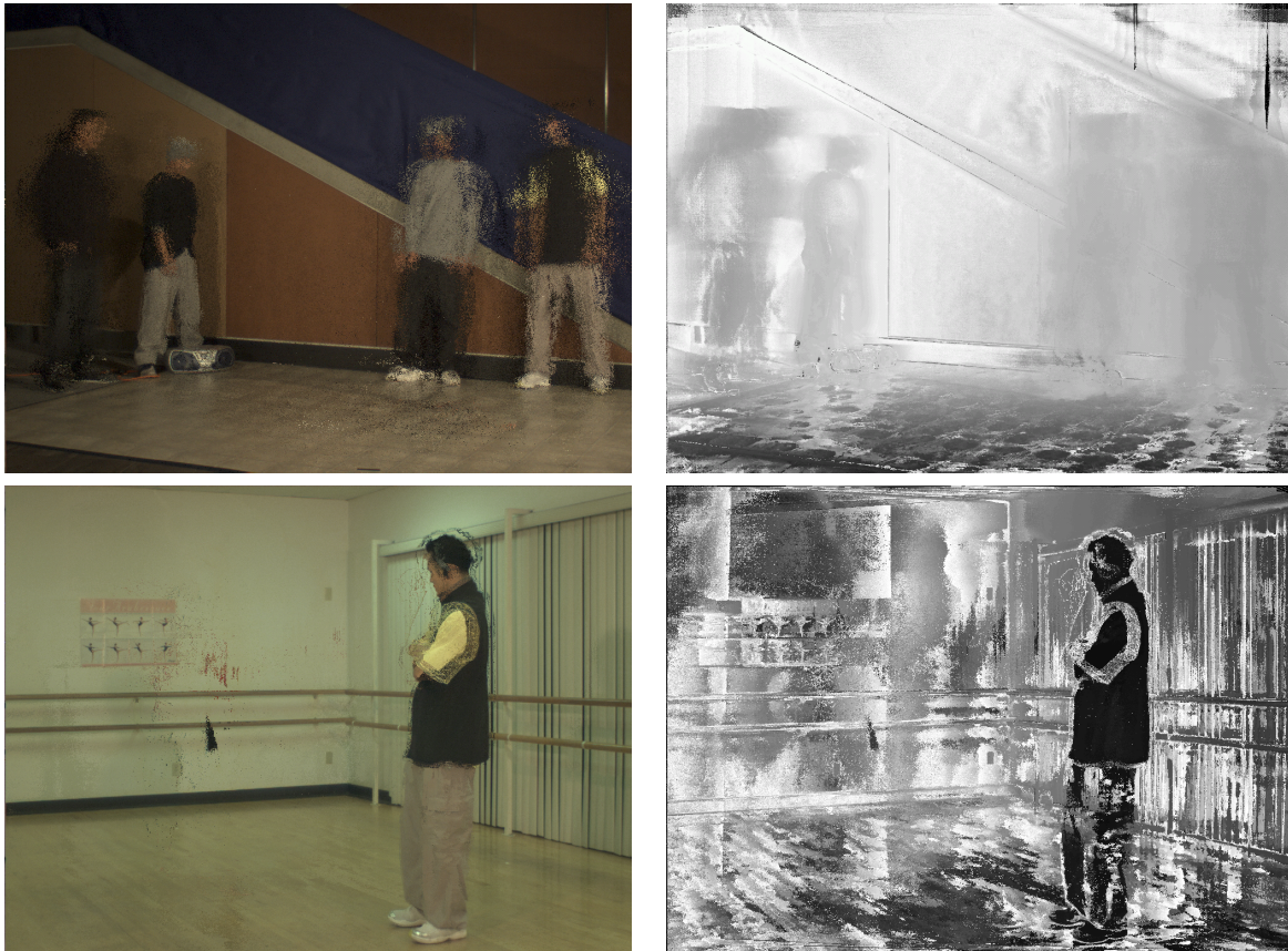
Figure 4.5: Background model (RGB Color on left and Depth on right) for the break-dancer and ballet sequences ((Zitnick et al., 2004)). Both results were obtained using 100 video frames and between 2 and 10 clusters (automatically selected per-pixel). Note that the people show up as “background” in regions where the true background is never visible.
