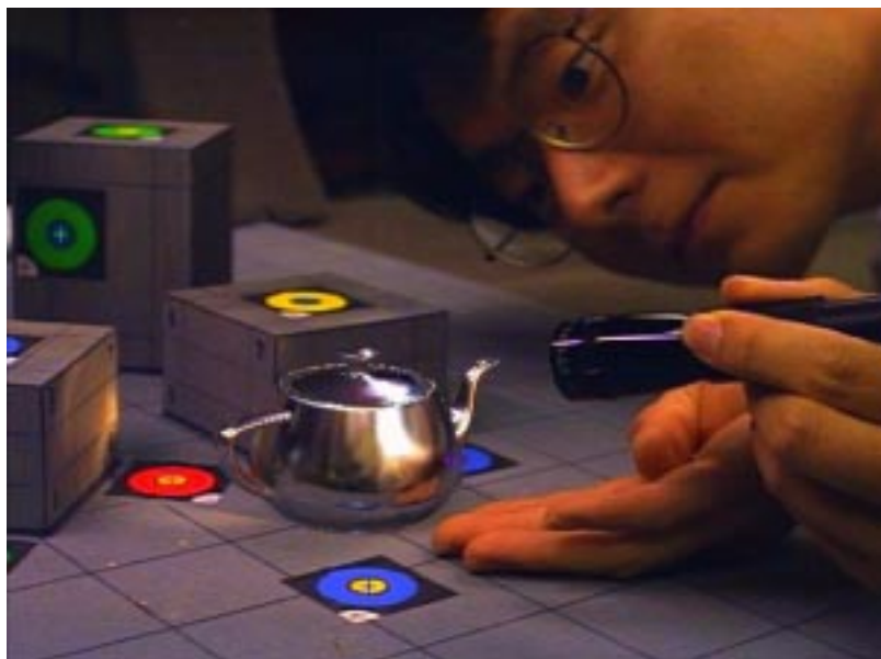
Figure 1.2: A tabletop AR environment in which a synthetic teapot reflects the real world that surrounds it. This effect is achieved by placing a reflective metal sphere at the appropriate location on the table, capturing the reflection map of that sphere by accurately knowing the projection of the sphere in the image, then rendering the reflection map onto the synthetic teapot. This image was created to demonstrate a vision-based tracking system developed at UNC [State96a] and described in Section 2.2.3.
