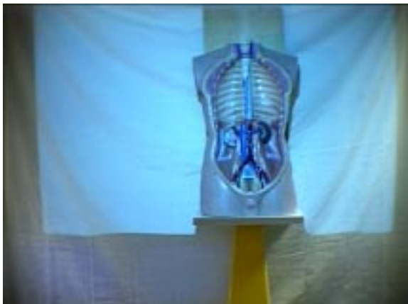
Figure 4.6: Scene of the experiment to measure landmark detection noise in an environment similar to the primary intended application, ultrasound-guided needle biopsy. A curtain hangs in the environment, yielding a non-planar, diffusely reflective surface. The medical training model in the foreground is life-size and has an exterior color of a fair-skinned human. Its interior consists of brightly colored models of interior anatomic structures.
