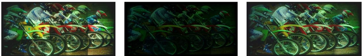
**Figure 8.8:** Digital photographs of a fifteen projector tiled display. Left: Before any correction. Middle: After photometric uniformity. Right: After constrained gradient based luminance smoothing.
