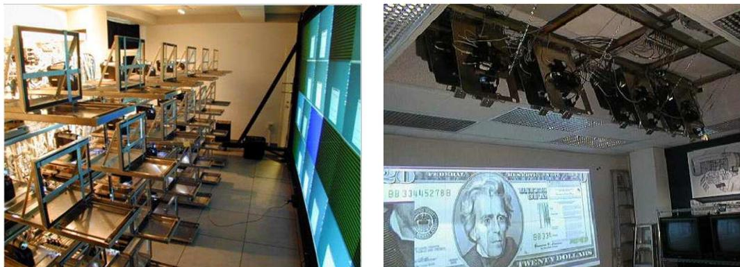
**Figure 2.11:** Left: Rear Projection System at Princeton University. Right: Front Projection System at University of North Carolina at Chapel Hill.
