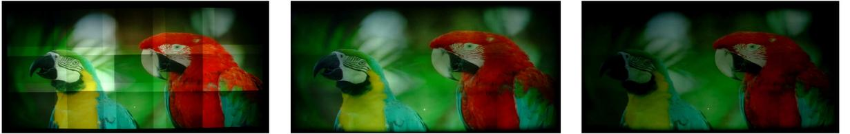
**Figure 8.9:** Digital Photograph of a fifteen projector tiled display. Left: Before any correction. Middle: Results with smoothing parameter of  $\lambda = 400$ . Right: Results with smoothing parameter of  $\lambda = 800$ .
