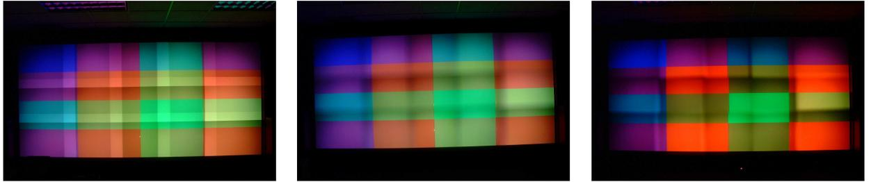
**Figure 1.6:** Fifteen projector tiled display at Argonne National Laboratory: before blending (left), after software blending (middle), and after optical blending using physical mask (right).
