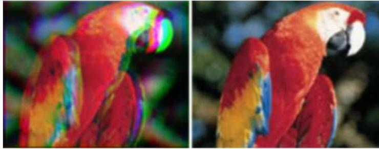
**Figure 2.5:** *The convergence problem of the CRT projectors (left) when compared with a light valve projector (right).*
