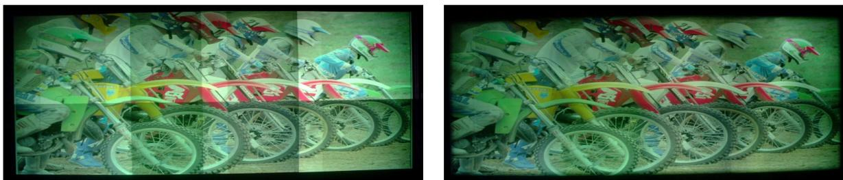
**Figure 8.11:** Digital photograph of eight projector tiled display showing the result of our scalable algorithm. The display luminance function for the left and right four projector configurations are reconstructed from two different orientations. The display luminance surface for the eight projectors is stitched from these. Left: Before correction. Right: After correction.
