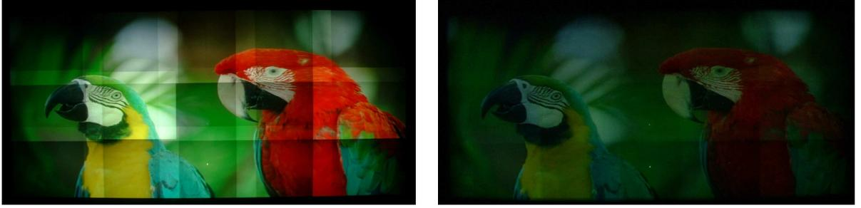
**Figure 1.7:** Digital Photograph of a  $5 \times 3$  array of 15 projectors. Left: Before Correction. Right: After absolute photometric uniformity (Matching only luminance).
