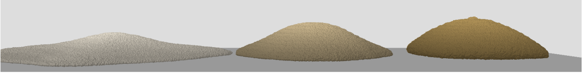
Figure 5.4: Three stable piles with friction coefficients \alpha = 0.3, 0.5, and 0.7, respectively. Lower friction leads to flatter piles.
