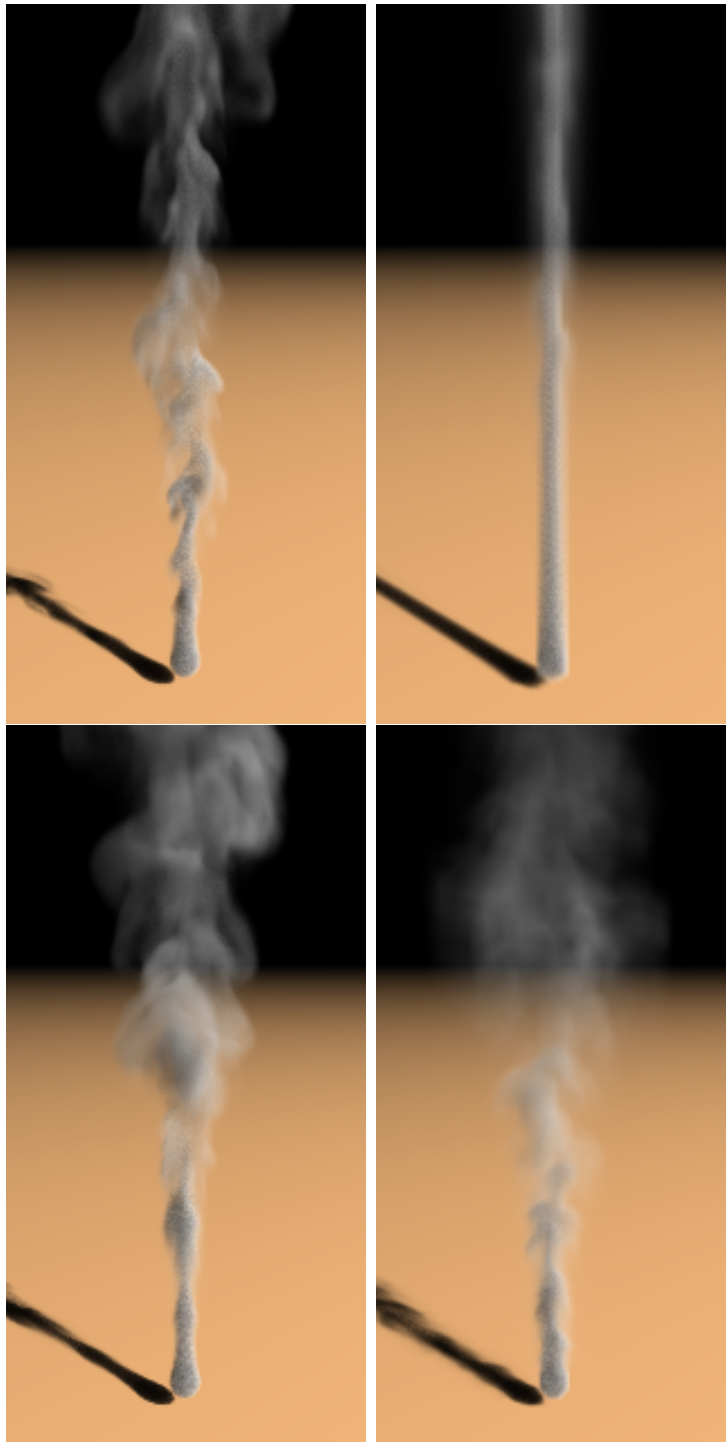
Figure 3.6: Smoke rising from a small density source, simulated with (a) the turbulence model, (b) low-resolution simulation only, (c) reference simulation on a 4\times refined grid, and (d) vorticity confinement on 2\times refinement.
