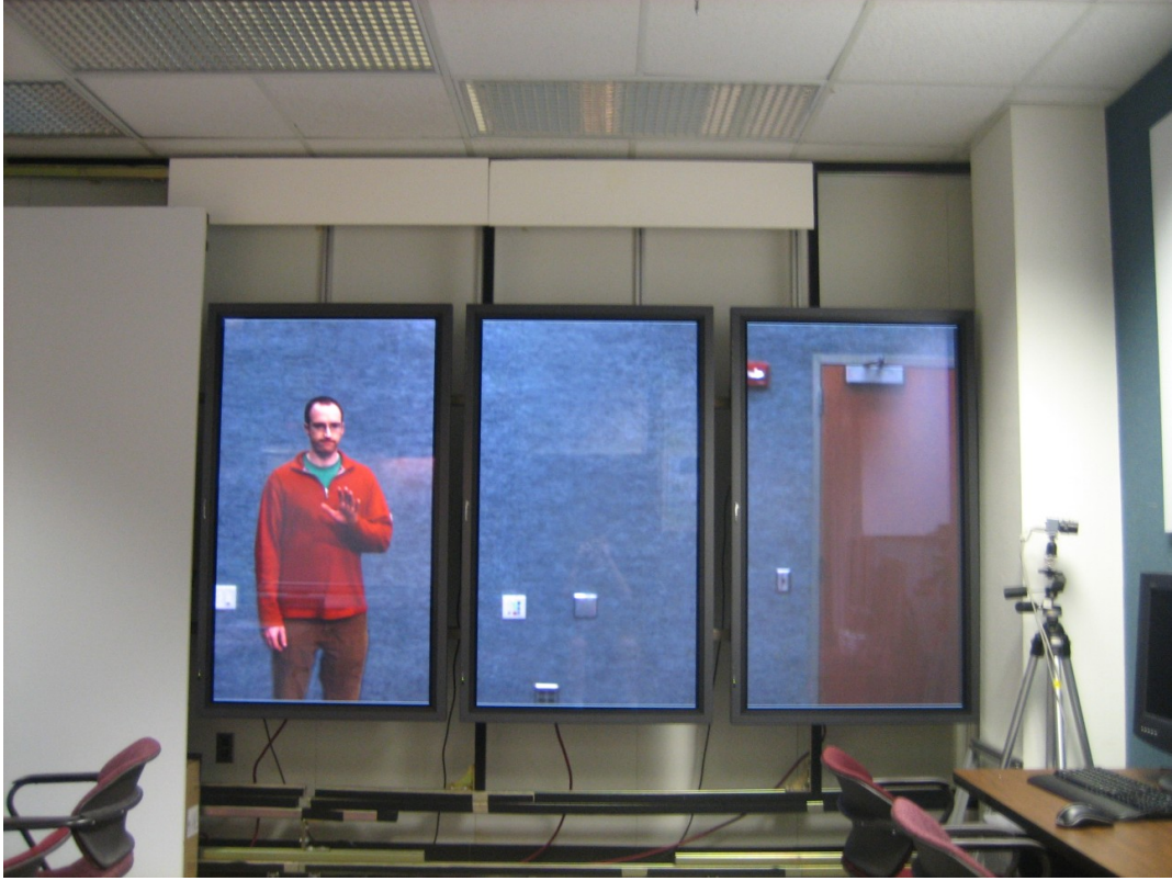
Figure 4.21: A photograph of video silhouette imagery shown on the telepresence wall displays.
