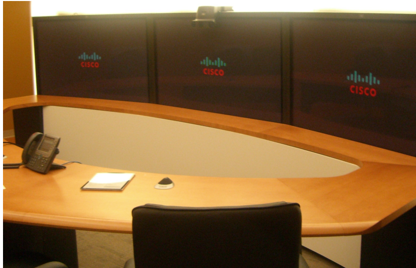
Figure 2.2: A side view of a Cisco Telepresence 3000 system. Three HD cameras are located in the cluster in the front-top of the central display. The placement of the cameras partially obscures the top of the screen but improves eye contact by reducing the parallax between the camera and the displayed remote users.
