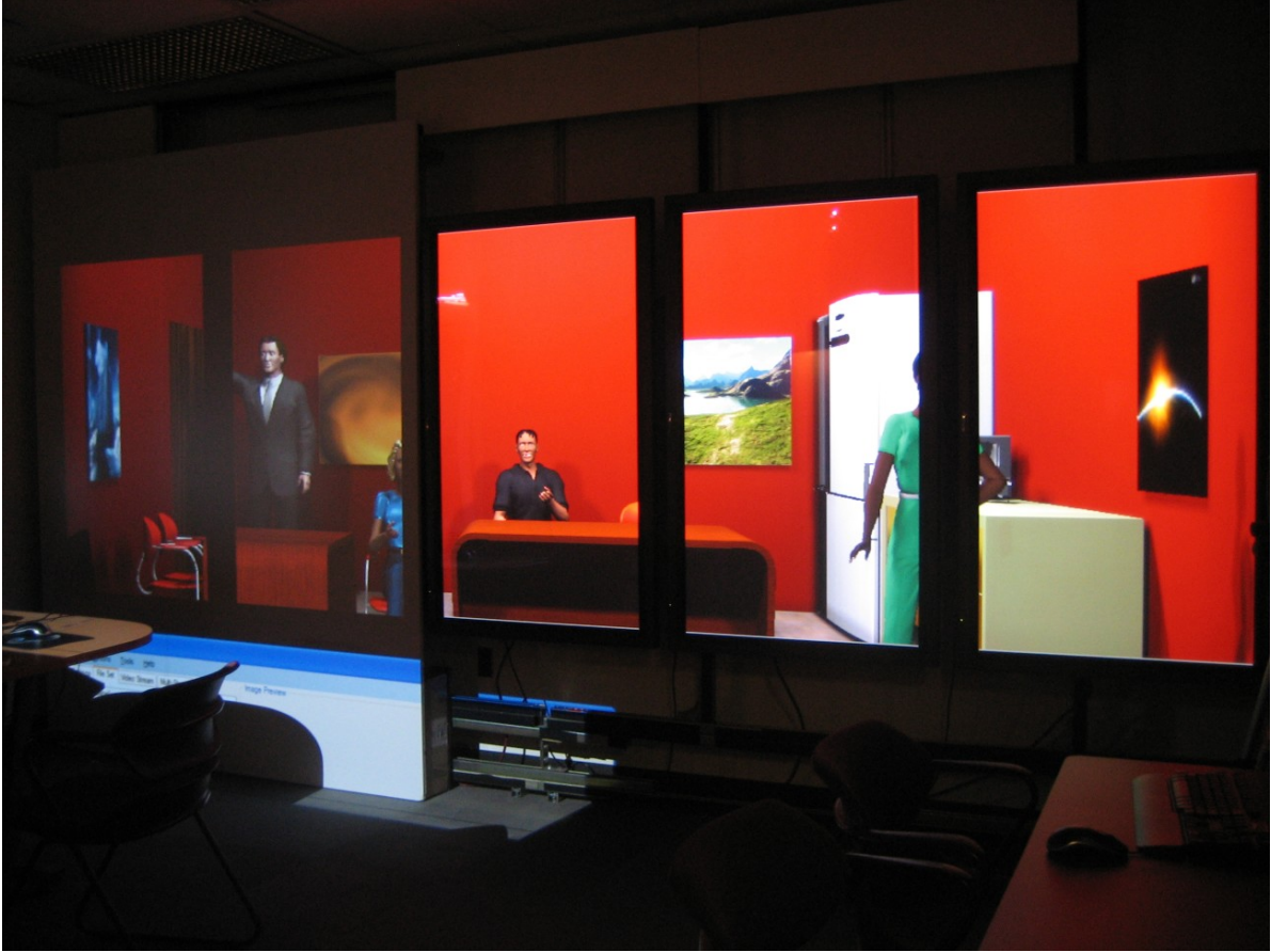
Figure 4.16: Telepresence wall display with flat panels and projected imagery showing a DDC image of the synthetic scene.
