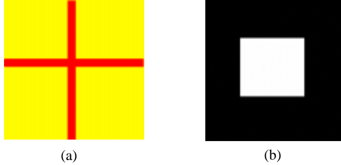
Figure 4-10. Texture (a) and depth map (b) associated with a relief texture of a quadrilateral with a deep box at the center. Black represents zero displacement and white represents deep unit displacement.
