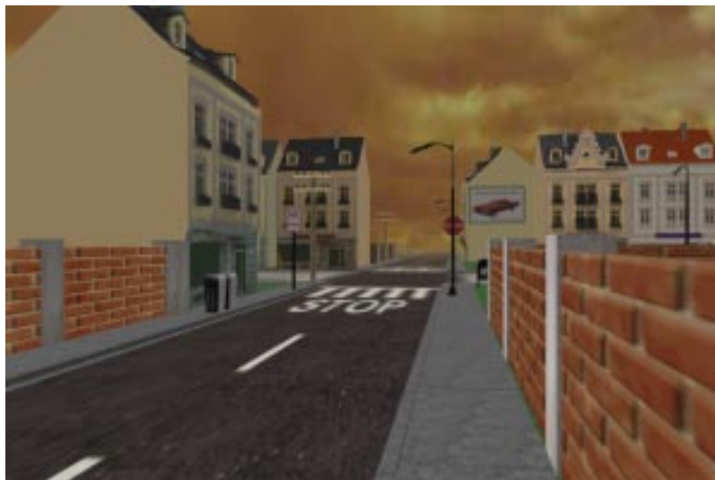
Figure 1-2. Same view as in Figure 1-1 rendered using relief texture mapping. Notice the bricks standing out and the protruding dormers.
