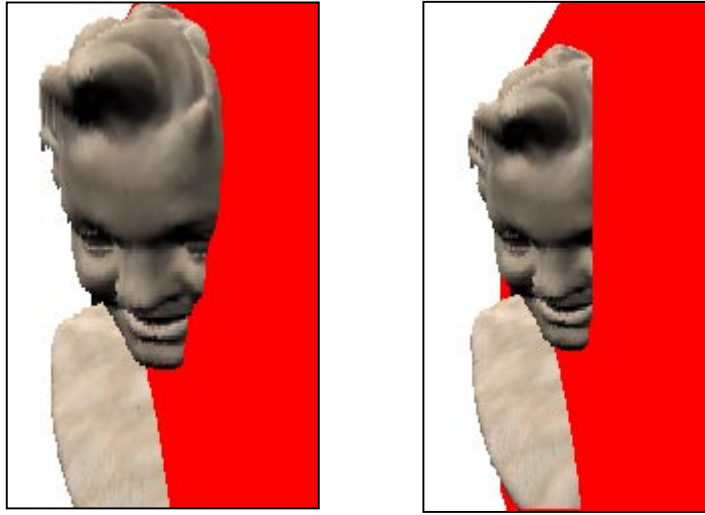
Figure 5-20. Relief textures rendered with z-correction using 8 bits to represent \Delta z_{screen} . The image to the left is virtually indistinguishable from its 32-bit counterpart. Occlusion errors start to happen as the screen-space delta values fall outside of the range appropriately covered by the available bits (right).
