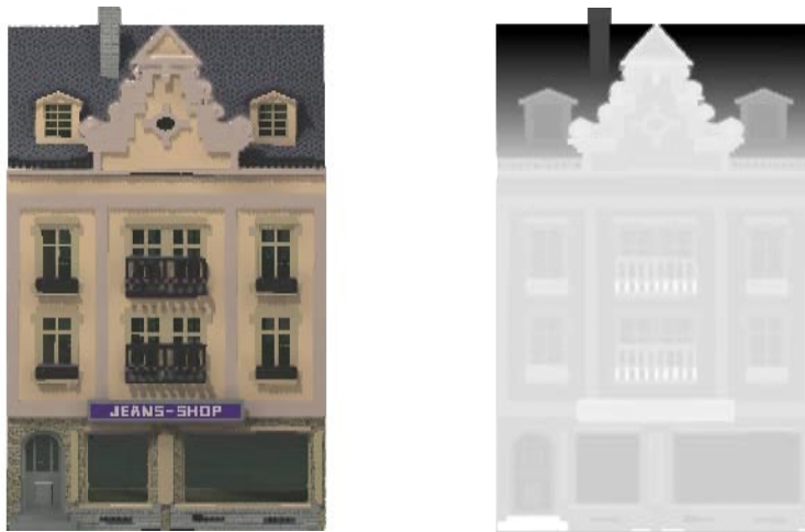
Figure 3-3. Color image (left) and depth map (right) associated with a relief texture. Darker regions in the depth map indicate more distant surfaces.
