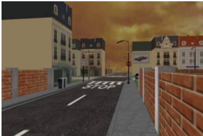
Figure 1-1. Town rendered using conventional texture mapping. Each façade and brick wall is represented by a single texture.
