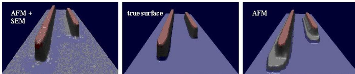
Figure 10-19: Comparison of the surface reconstructed by optimization of the likelihood computed from the AFM image and the SEM image (left), the true surface (center), and the surface found by grayscale erosion of the AFM image(right).
