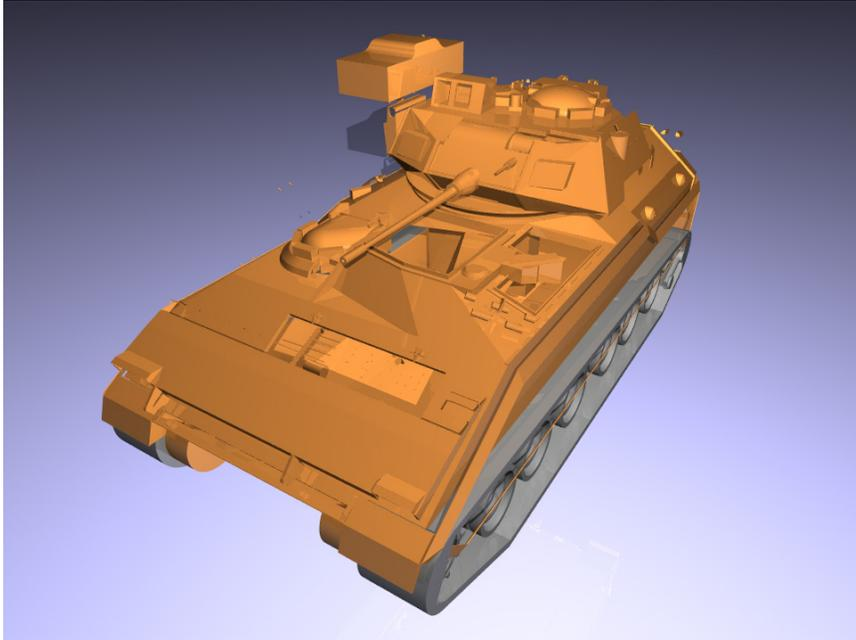
Figure 1.1: Bradley Fighting Vehicle: *This image shows a view of the Bradley Fighting Vehicle. This model has over 8,500 solids generated entirely using Boolean operations.*
