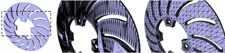
Figure 1.10: Remeshing: *The left image shows a brake hub model, which has many “skinny” triangles with poor aspect ratios (center image). We used our algorithm to compute an improved triangulation of the model (right image). The original brake hub model has 14K triangles. Our algorithm took 1.85 secs to perform remeshing and generate a mesh with 7K triangles at a relative Hausdorff error of 1/32.*
