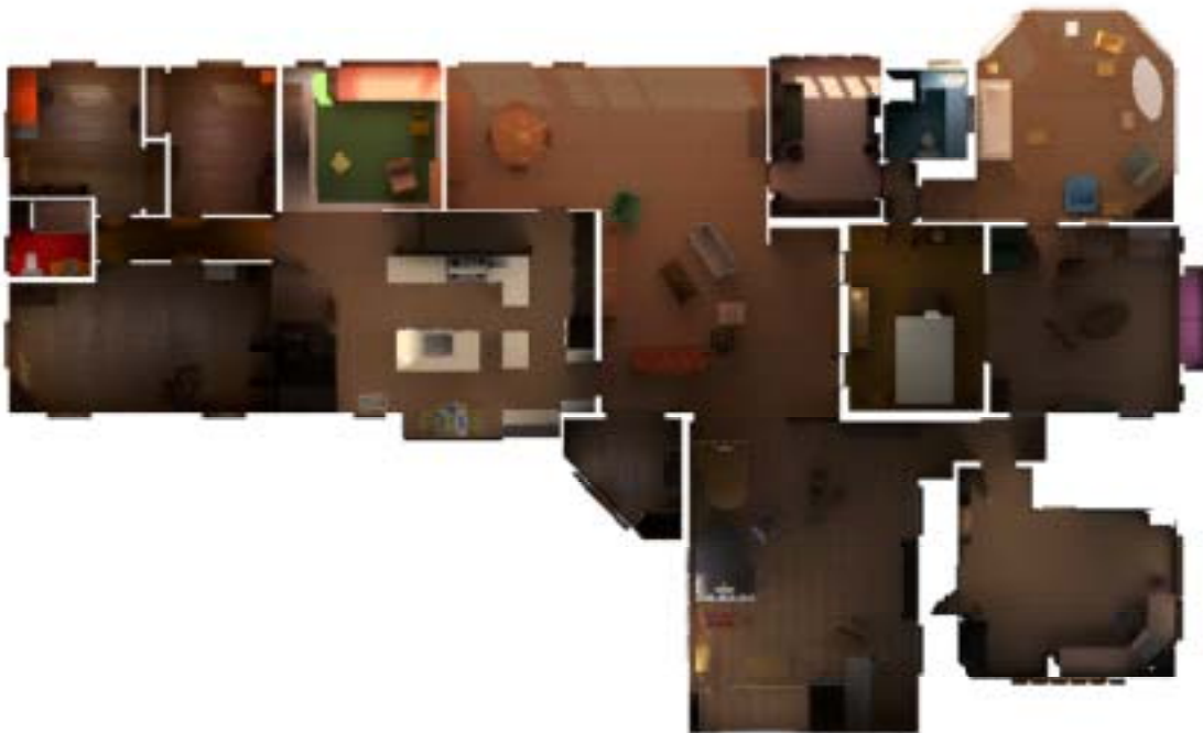
Figure 1.1: A model of a house containing approximately 274,000 triangles and 19 megabytes of high-resolution textures. Per-vertex colors are used to store a global illumination solution. Model courtesy of UNC Walkthrough group.
