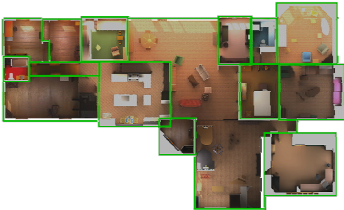
Figure 2.1: Cells and portals in a model of a house. The visible set within any given cell (outlined in green) can be reasonably approximated with the objects in that cell. To simplify processing, complex cells (such as the one in the center of the model) can be subdivided into smaller rectangles. Transparent portals such as doors and windows connect neighboring cells.
