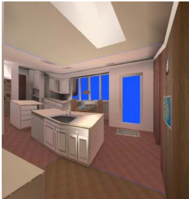
Figure 7.7: Example of perspective distortion caused by lack of depth parallax in impostors. The viewpoint is near the cell boundary in this image. Also note the color discontinuity between impostor and geometry.
