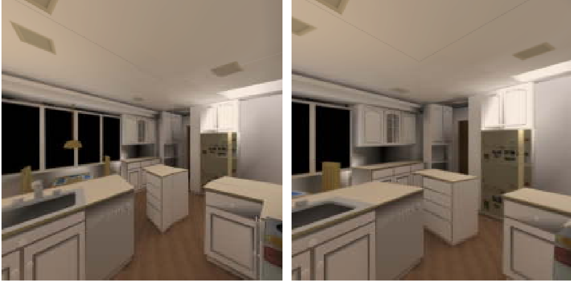
Figure 7.5: Popping artifacts can occur when the user moves from one cell to another. These two images were taken from the MPEGWALK system using flat texture-mapped quadrilaterals as impostors. Their respective viewpoints are roughly 2 inches apart with identical view directions. Note such differences as the stretching of the cabinet in the mid-lower image, the size and position of the refrigerator at left, and the dramatic change in both the size of the cabinet on the far wall and the visibility of the table beneath the black windows. Moreover, the orientation of the sink at lower right has changed significantly. All of these differences are due to perspective distortion arising from our choice of impostor representation in MPEGWALK. The popping artifact occurs when the distortion in the impostors changes abruptly and objects appear to jump and stretch from one image to the next.
