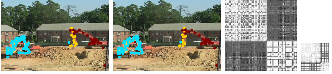
Figure 4.7: ( left 2 ) A sequence of two bulldozers moving independently, one of which moves articulately with its arm rotating around an axis. The color of a dot, red, blue or yellow, shows the segmentation result. There is one misclassification error which is the red dot on the forearm near the axis. Besides that, there are several outliers. ( right 2 ) The affinity matrices for 2-stage segmentations are shown. The row and columns are rearranged based on the segmentation.
