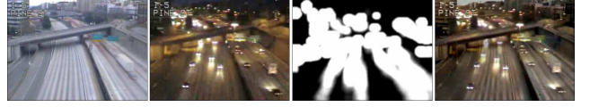
Fig. 3. Enhancing traffic video. A high quality daytime and a low quality nighttime video frame, the importance image obtained after processing, and the final output of our algorithm.
