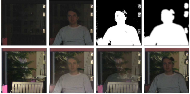
Fig. 2. Enhancing a dynamic scene. (Top row) A low quality nighttime reference, and with a foreground person, a simple binary mask, the importance image obtained after processing. (Bottom row) A high quality daytime snapshot, the final output of our algorithm, compared with averaging and blending pixel intensities.
