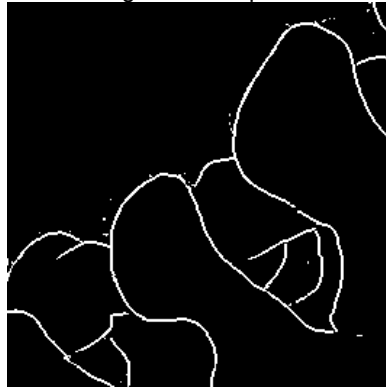
Resultant depth edges detected by NPR camera
