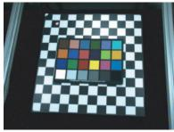
Figure 6. The geometric and photometric calibration patterns, as seen from one of the eight cameras. The patterns shown together here are actually used separately for geometric and photometric calibration.
