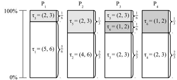
Figure 5: EDF-os task assignment for Ex. 1.
