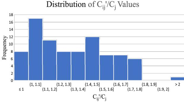
Fig. 4: Histogram showing the distribution of  $\frac{\text{time SMT is in use}}{\text{solo execution time of shorter job}}$ , i.e.  $\frac{C'_{i:j}}{C_j}$ , when using the definitions in our data driven model. Based on data from [14].
