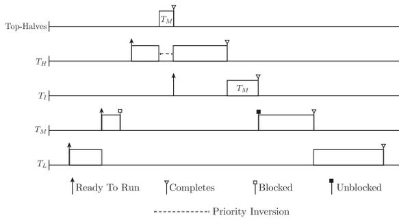
**FIGURE 1:** Fixed-priority assignment when an I/O device is used by a single thread.
