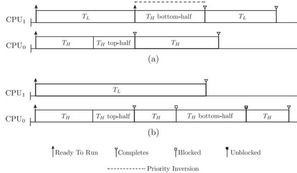
**FIGURE 6:** (a) Priority inversions may occur when a bottom-half is co-scheduled with the thread from which it is inheriting priority. (b) Deferring execution of the bottom-half until its owner relinquishes a CPU prevents the priority inversion.
