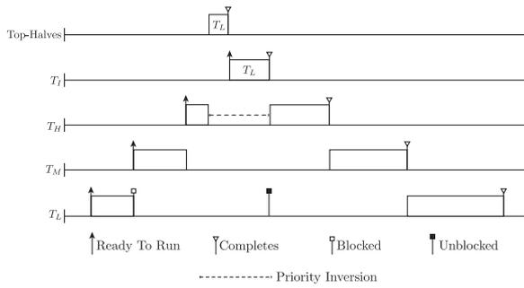
**FIGURE 3:**  $T_H$  may suffer a bounded priority inversion when  $T_I$  processes a bottom-half for  $T_L$ .
