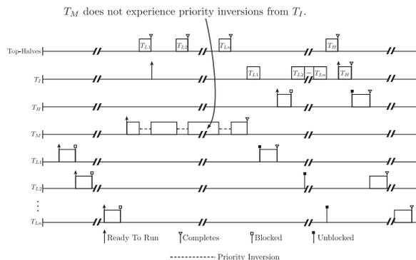
**FIGURE 5:**  $T_I$  with a dynamic priority.  $T_I$  is only scheduled with a high priority when the device is in use by  $T_H$ .
