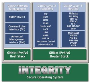
The GateD family of routing and switching software supports all requisite Layer 2 and Layer 3 protocols and provides a processorneutral, comprehensive control plane and data plane solution for next-generation carrier devices.
