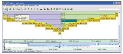
The TimeMachine debugger interface is integrated with advanced analysis tools such as the PathAnalyzer, which shows your call stack over time.
