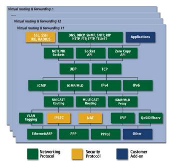
INTEGRITY's TCP/IP stack provides a comprehensive set of industry standard protocols in a high-performance, scalable stack.
