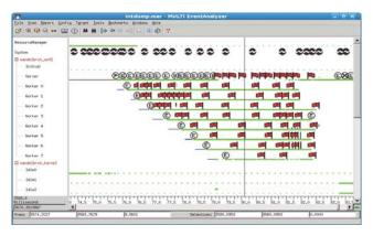
Any event displayed in the EventAnalyzer view window can be selected for debugging with a single click, opening a debug window showing that event's source code, ready to debug.
