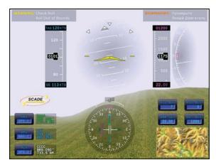
INTEGRITY supports 3D graphics—including OpenGL via leading-edge embedded products from ALT Software.
