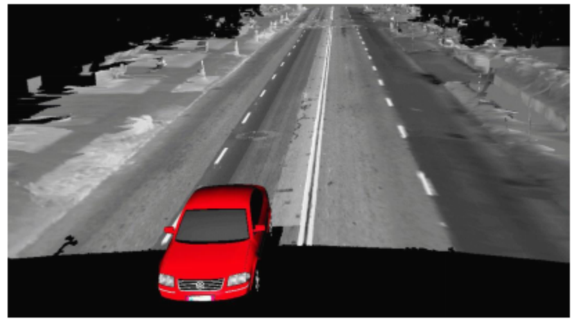
Figure 2. Visualization of the scanning process: the LIDAR scanner acquires range data and infrared ground reflectivity. The resulting maps therefore are 3-D infrared images of the ground reflectivity. Notice that lane markings have much higher reflectivity than pavement.
