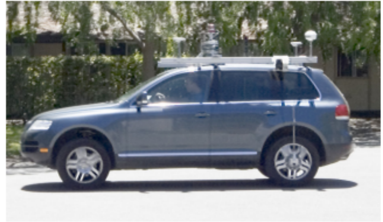
Figure 1. The acquisition vehicle is equipped with a tightly integrated inertial navigation system which uses GPS, IMU, and wheel odometry for localization. It also possesses laser range finders for road mapping and localization.
