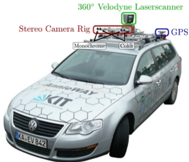
Figure 1: The standard station wagon is equipped with color stereo camera, grey stereo camera, Velodyne Laser Scanner, and GPS system.
