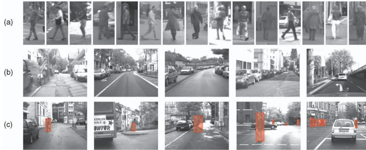
Figure 8: Daimler pedestrian detection benchmark data set: (a) Pedestrian training samples, (b) nonpedestrian training images, (c) test images with annotations. Source from [9].
